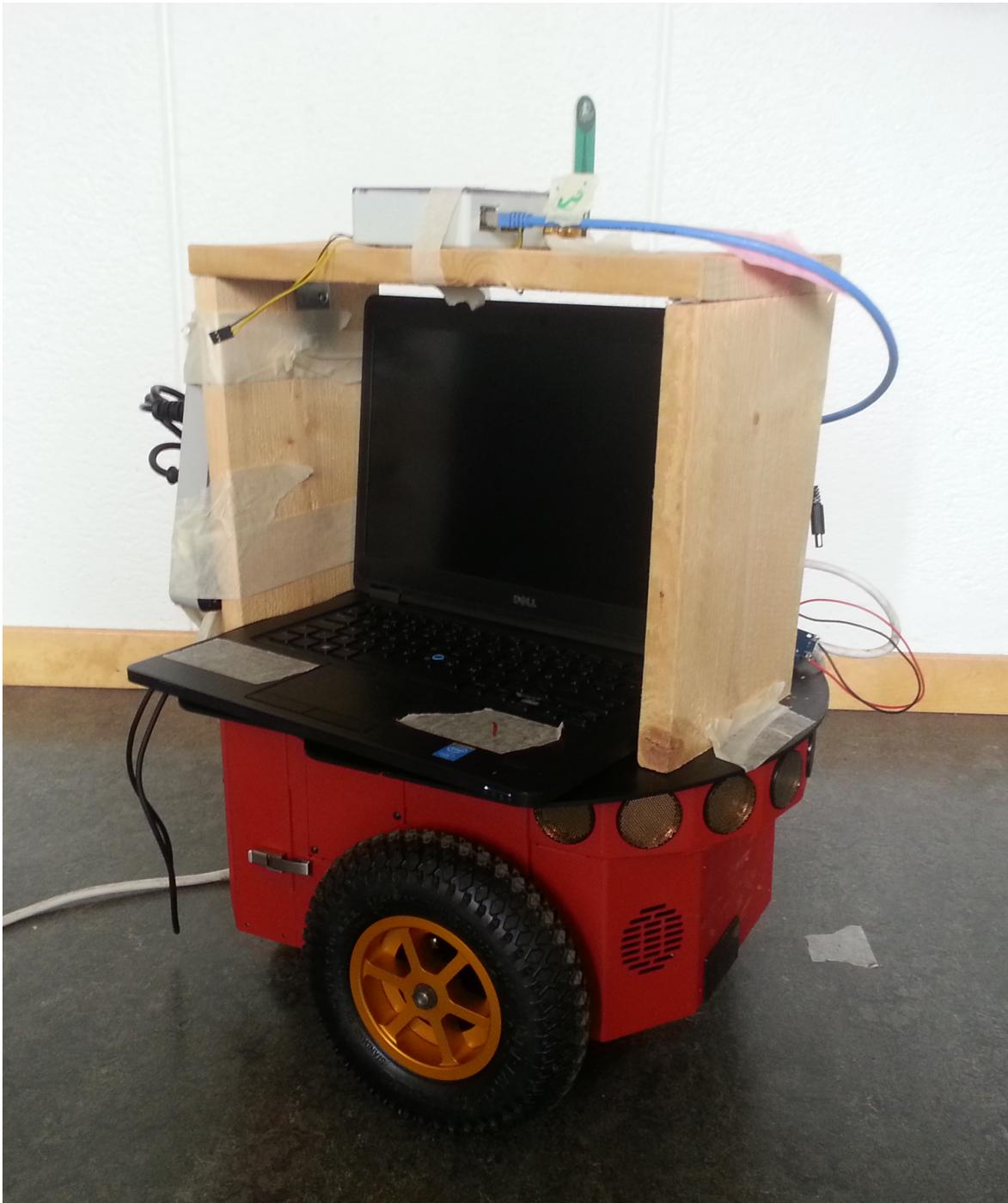
**Figure F.1:** Picture of the actual relay construction used. The RCM and node (laptop computer) mounted upon the Pioneer robot. There is a battery behind the laptop feeding the RCM power and thus allowing the relay to run without a power cord connected to it.
