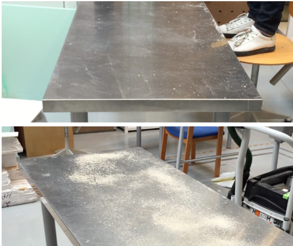
Figure 79 The result of blowing from above. Top: blowing perpendicular to the table. Bottom: same test but with a dirty table 3m away (horizontally).
