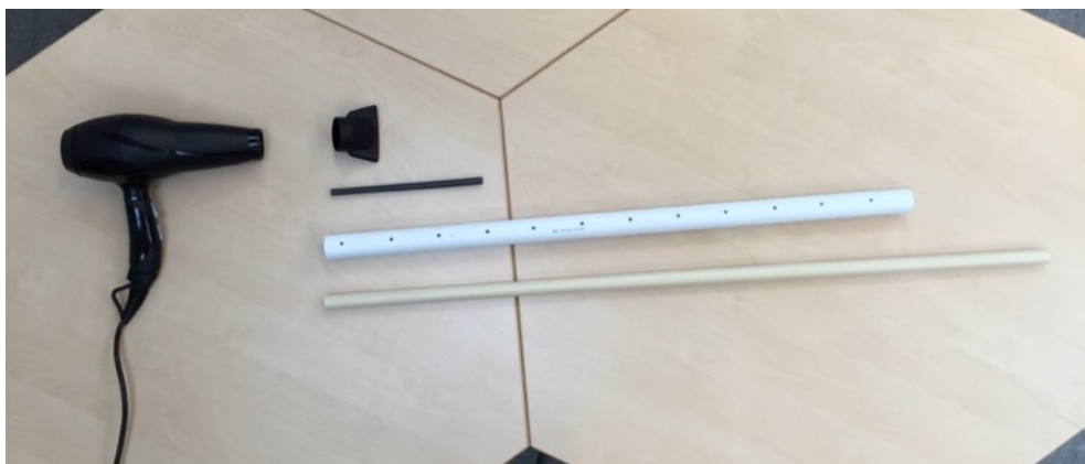
Figure 8 Materials used to create different nozzles - add-on nozzle included with the blow dryer, straws and PVC pipes in different sizes.
