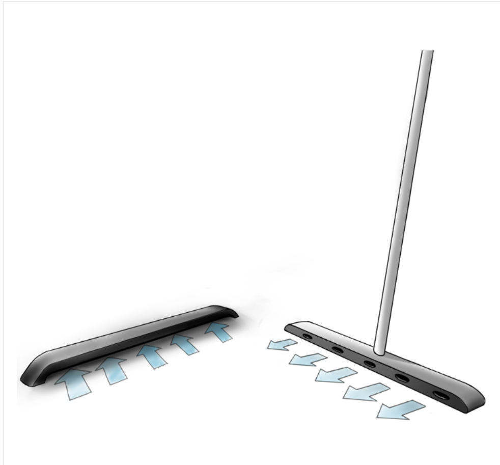
Figure 56 SUR - a suction device put beneath furniture and a stick blower.
