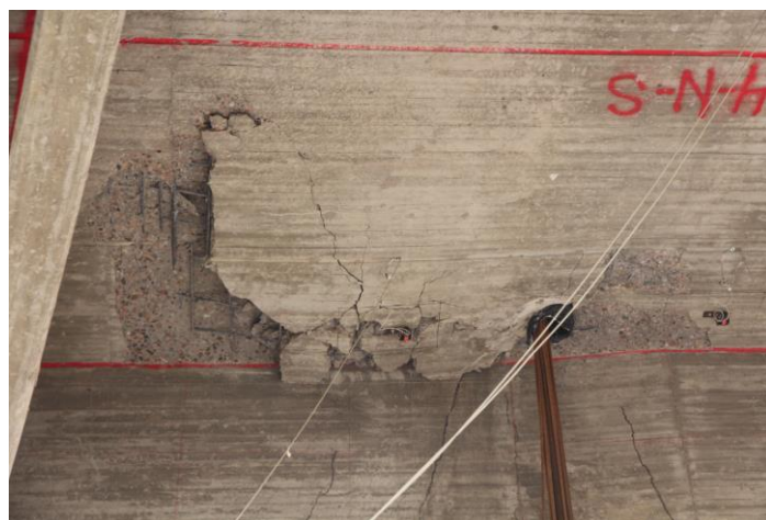
Figure 7: Bottom view of the slab showing punching failure occurred at the further loading plate.
