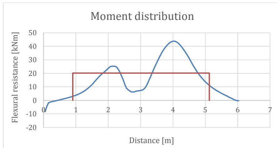
Figure 31: Moment distribution along critical cross section (blue line) and distribution width with average bending value (red line).
