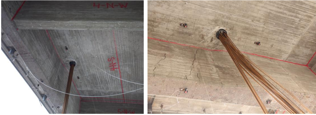
Figure 5: Bottom view of the slab showing the location of the loading points.
