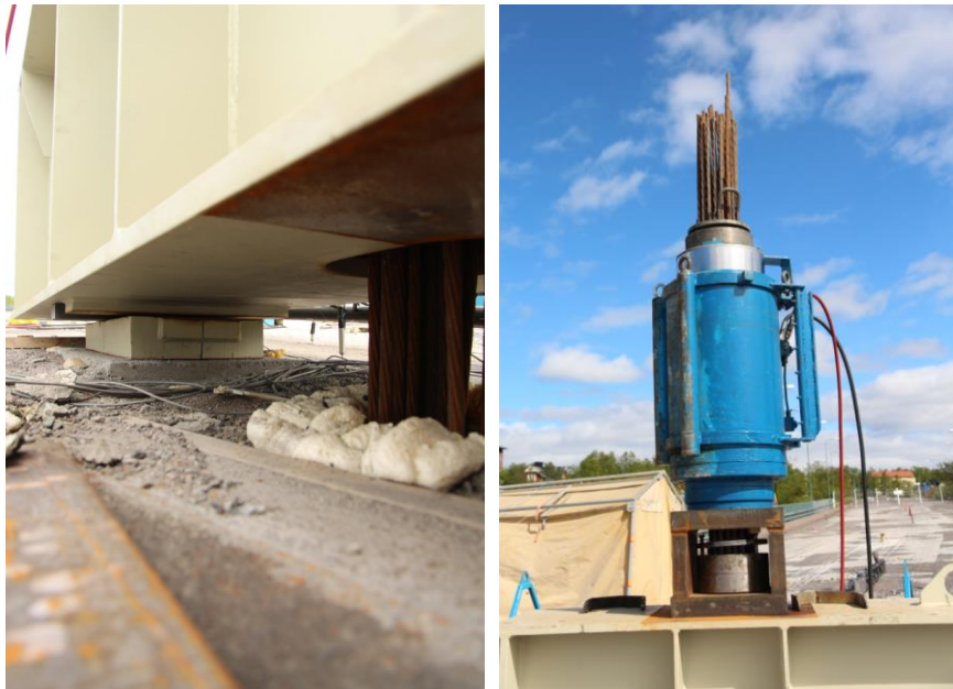
Figure 6: Devices installed above the slab: Closer loading area and stiff steel beam which connected the two loading plates (left) and hydraulic jack (right).
