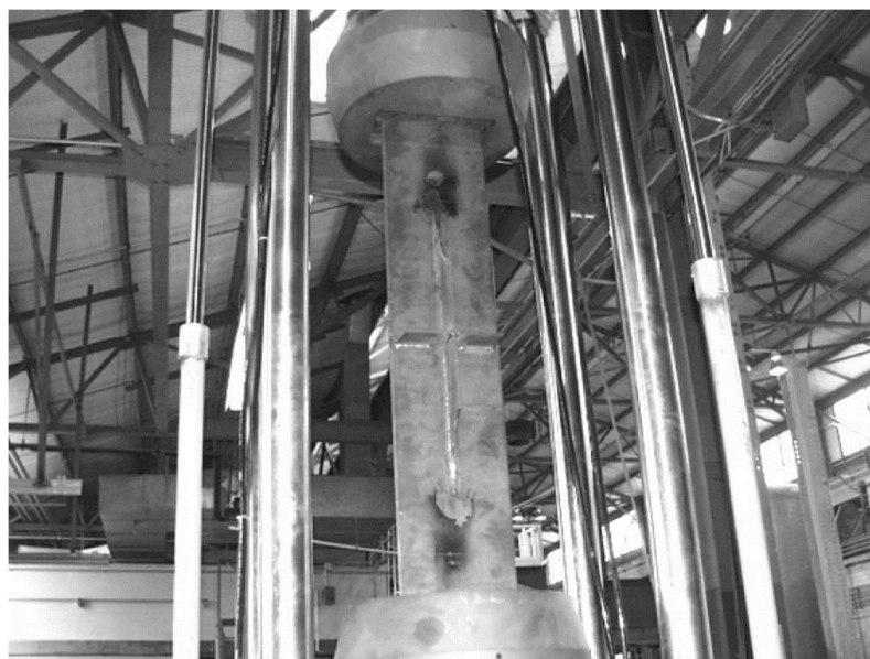
Figure 3.3 Typical fatigue experimental setup (Spadea & Frank, 2002).
