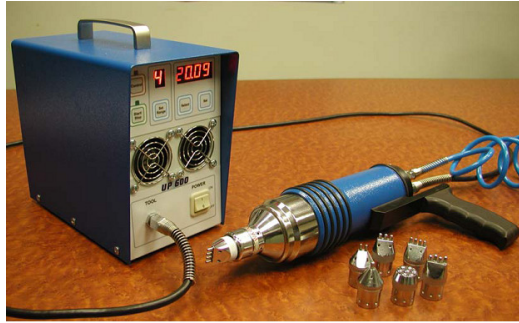
Figure. 23-Basic ultrasonic peening system for fatigue life improvement of welded elements and structures. (SINTES-Technology and Equipment for Ultrasonic Impact Treatment (UIT/UP), 2015).
