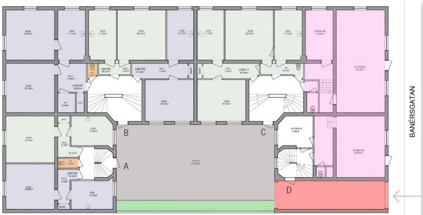
Figure 14 Actual first floor (ground floor), with brick walls. Marked in orange the shared toilets, in pink the two private storages facing the street, in blue and green the different typology of apartments, in red the main entrance, and in grey the common patio
