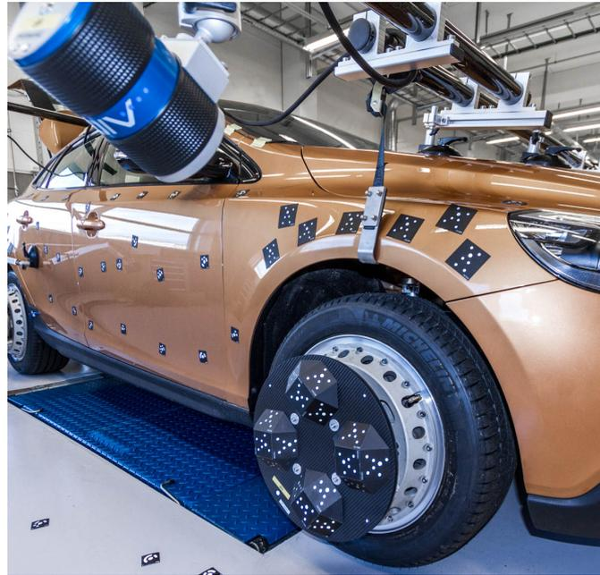
**Figure 4.21:** AICON WheelWatch camera system
