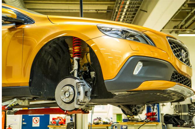
**Figure 4.16:** Modified Volvo V40 struts installed on vehicle
