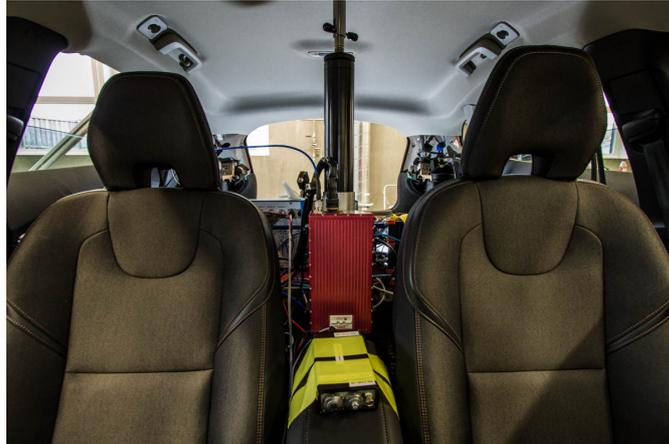
**Figure 4.20:** Inertial measurement unit mounted in vehicle
