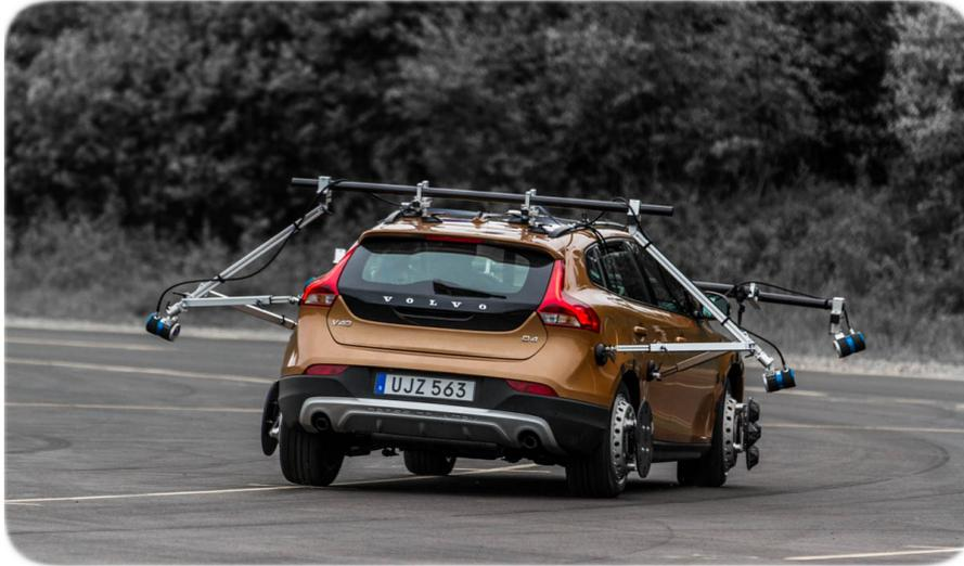
**Figure 4.22:** Vehicle performing linear range maneuver while instrumented with measurement equipment.
