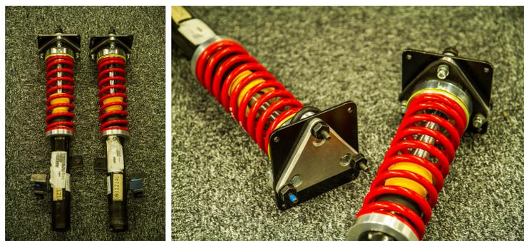
**Figure 4.15:** Modified Volvo V40 struts and camber adjustment plates
