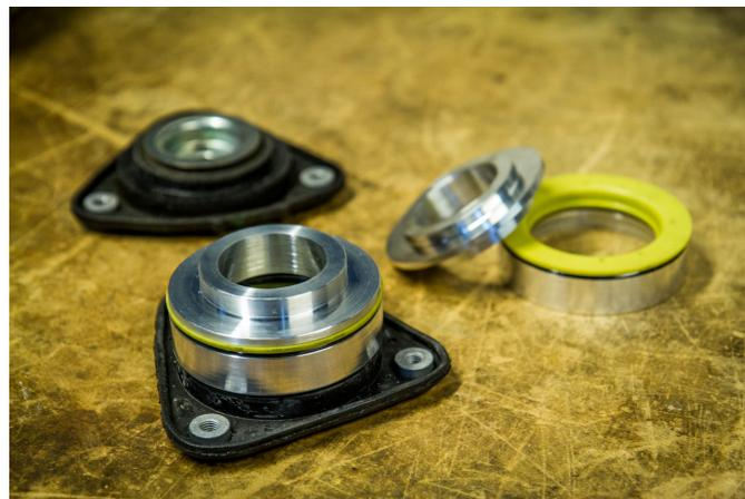
**Figure 4.14:** Machined strut bearing assembly
