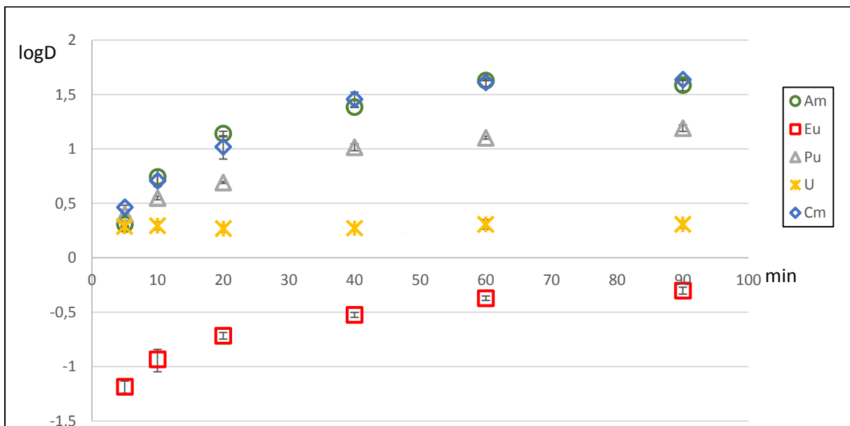
Figure 4.1.1. Logarithmic distribution ratios over time for uranium, plutonium, americium, curium and europium using octanol as diluent.
