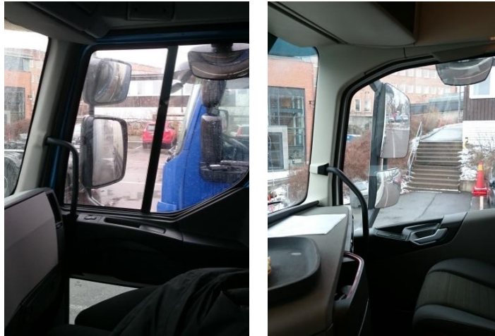
FIGURE 17: ILLUSTRATION OF THE EXTRA WINDOW IN THE VOLVO FE TRUCK
