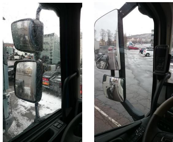
FIGURE 16: DIFFERENCE IN SPACE BETWEEN A-PILLARS & MIRRORS—VOLVO FE (LEFT) AND VOLVO FH (RIGHT)
