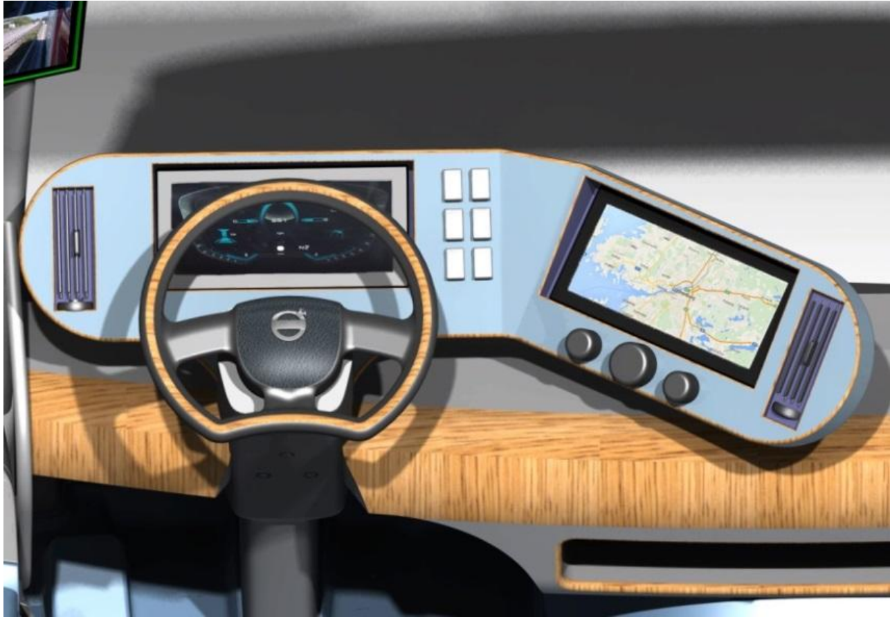
FIGURE 52: ADJUSTABLE UPPER INSTRUMENT PANEL FOR THE VOLVO FE TRUCK
