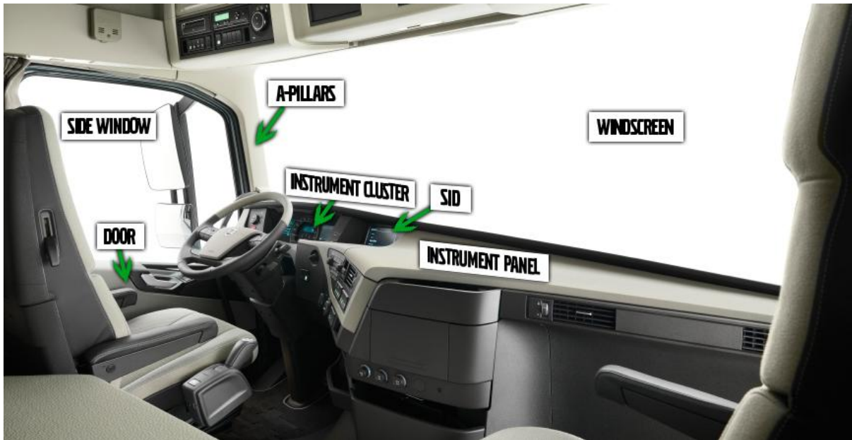
FIGURE 1: ILLUSTRATION OF THE COMPONENTS IN THE CURRENT VOLVO FH INCLUDED IN THE SCOPE
