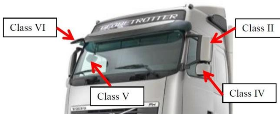
FIGURE 13: DIFFERENT MIRROR TYPES ON VOLVO FH TRUCK (Fagerström & Gårdlund, 2012)
