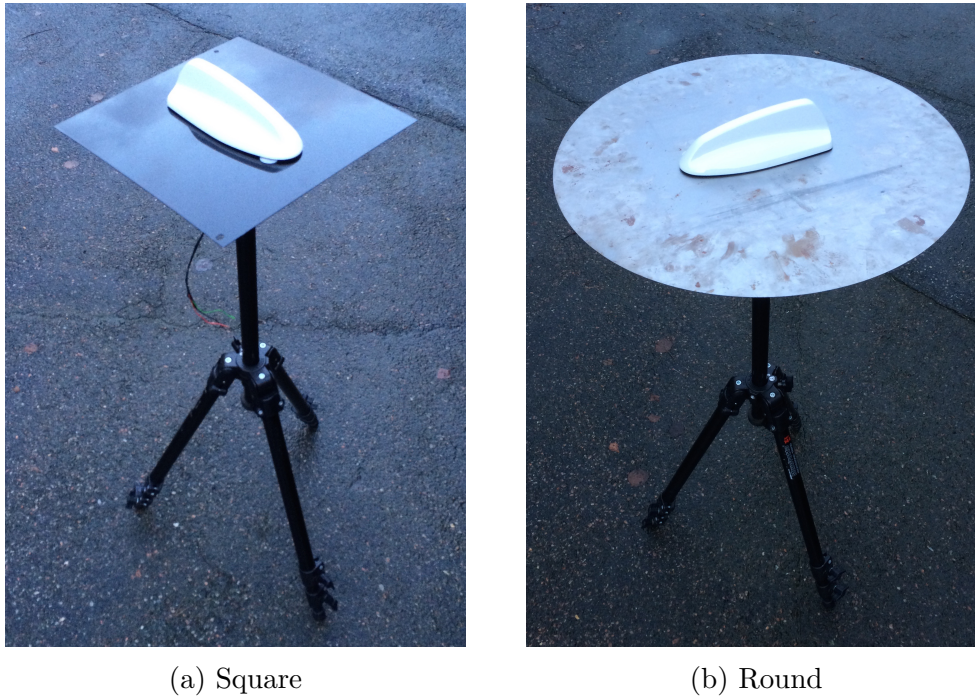
Figure 3.4: The two used ground plane. The square ground plane, figure 3.4a, is 30 \times 30 cm, and the round ground plane, figure 3.4b, is 50 cm in diameter.
