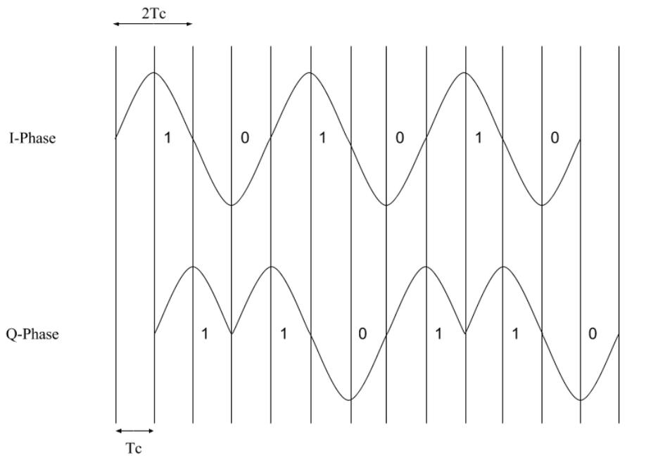
**Figure 2.4:** Modulated chip sequences
