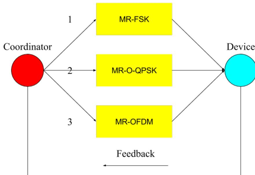
**Figure 5.2:** Dynamic mode switching mechanism
