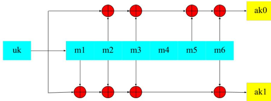
Figure 4.1: convolutional encoder
