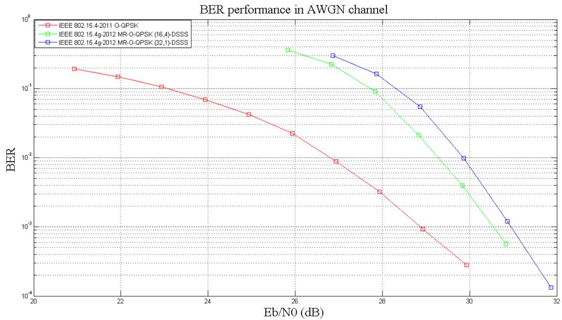
**Figure 4.5:** BER performance in AWGN channel
