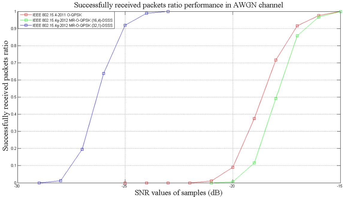
**Figure 4.4:** Successfully received packets ratio performance in AWGN channel
