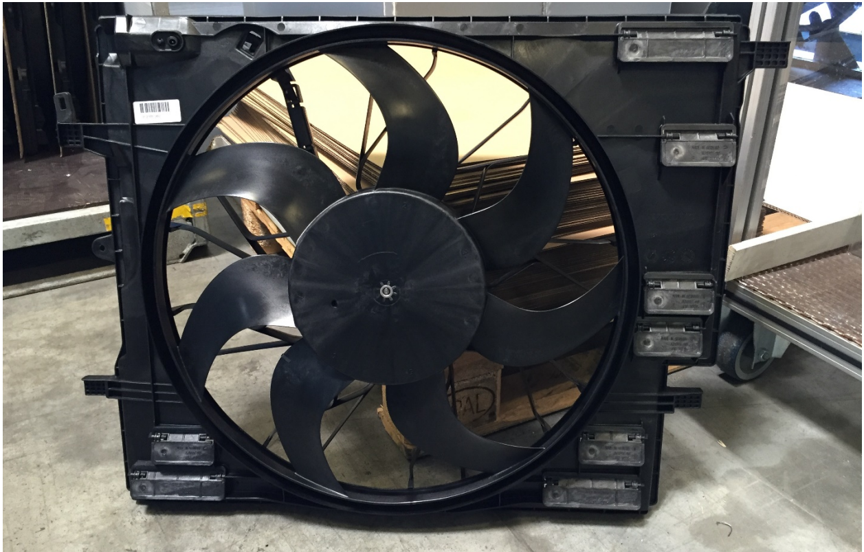
Figure 3. A complete cooling fan. An electrical motor in the center of the module drives the rotation of the fan.
