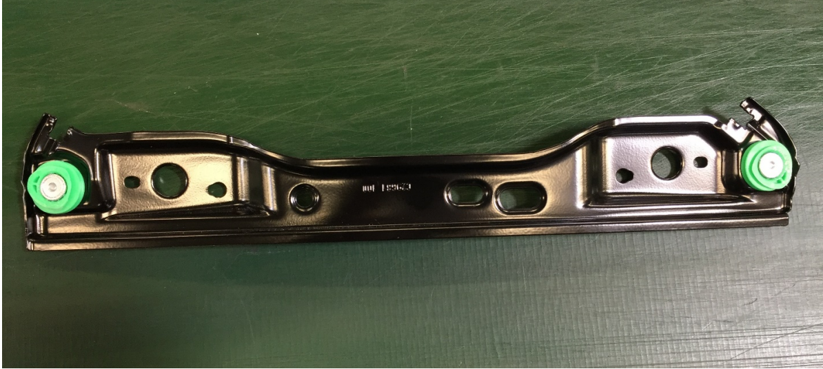
Figure 1. An assembled rail. The two pulleys on each end of the rail guide the wire that enable the window regulation system.
