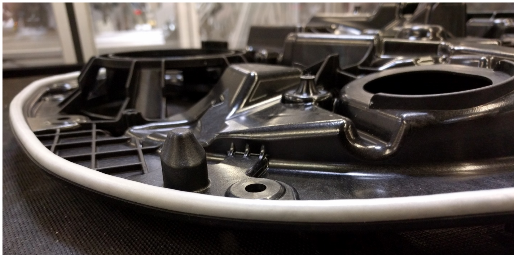
Figure 12. A close-up of the plate and the sealant. The sealant is the substance that can be seen on the edge of the plate.
