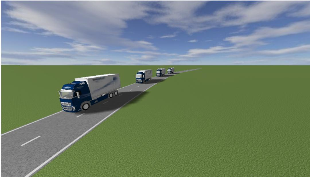
**Figure 4.2:** The evaluated platoon in PreScan environment with four HDVs with three following vehicles and one leading vehicle. The width of the lane is 3.5 meters and each HDV has a longitudinal speed of 20 m/s.
