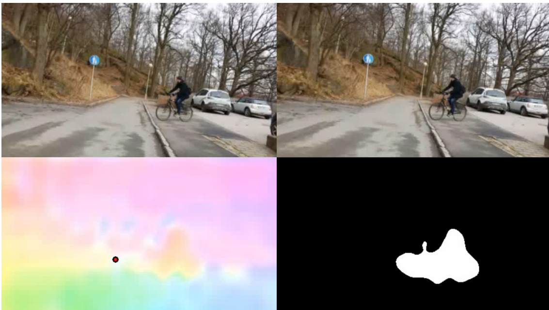
Figure 5.1: An illustration of when the algorithm gives a satisfactory result. Top left and top right shows frame one and frame two, respectively. Bottom left shows the optical flow field as calculated by PCA-Flow, where the FOE has been marked with a red circle with black border. Bottom right shows the segmentation result when using an angle threshold of \pi/2 . As the frames are subsequent in the video used, the frame jump in this example is 1.
