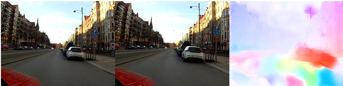
Figure 2.3: An example of how optical flow can be visualized. The left image is the first frame, and the middle image is the second frame. The right image is a visualization of the resulting optical flow, as calculated by the EPPM algorithm [1].
