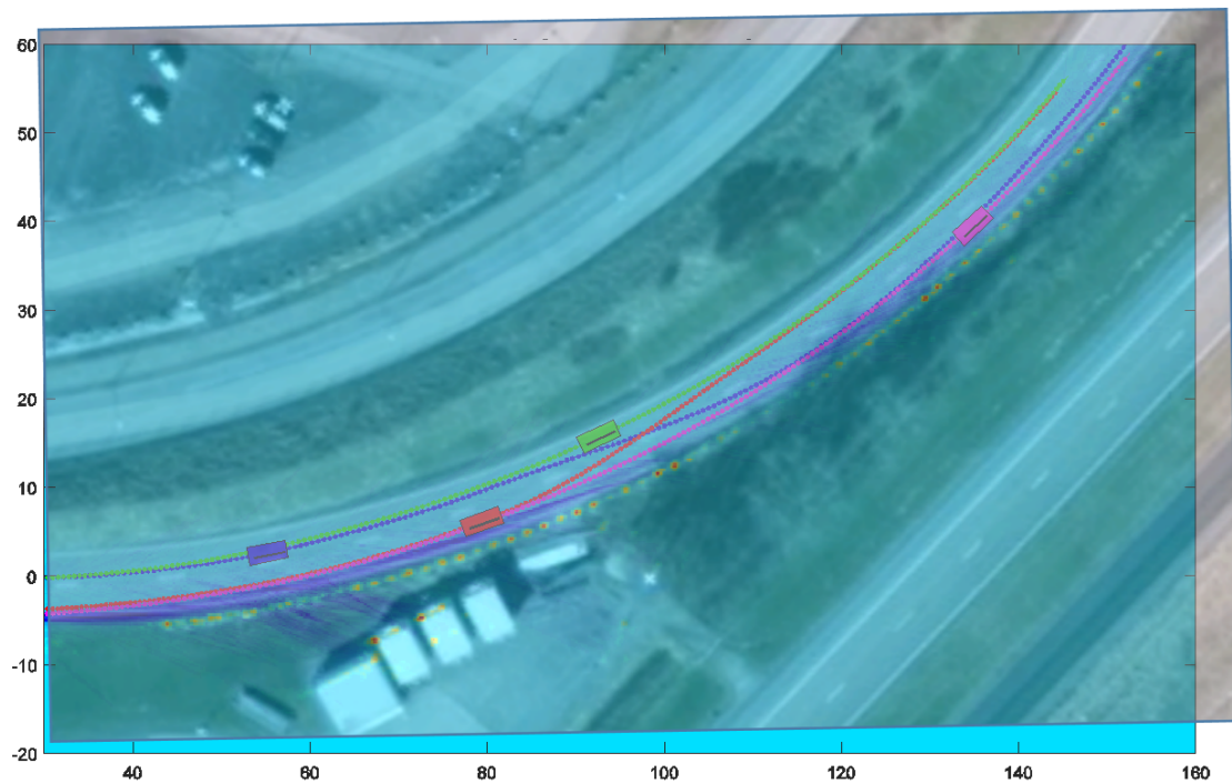
Figure 7.3: The 2D projected OGM from Figure 7.2 and the real test scenario from Figure 2.4 are aligned, and the OGM is set transparent. The alignment isn't perfect, but the dots of high probability of occupancy in the OGM correspond to the poles in the guardrail and the corners of the small houses.
