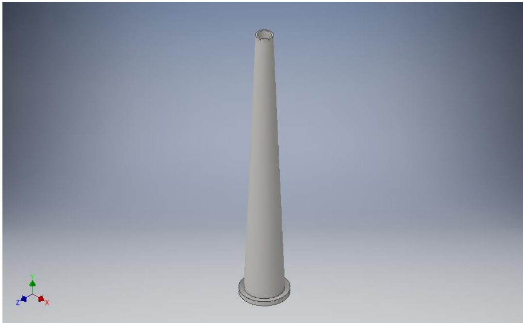
Figure 4.1 Simplified model of the tower used during the preliminary study.
