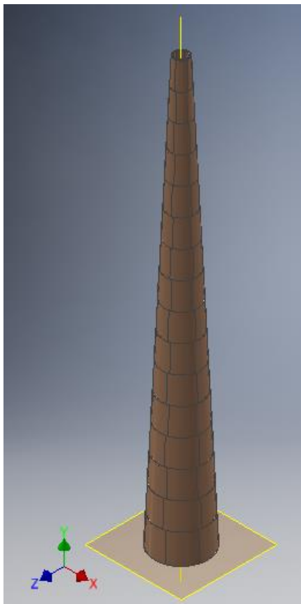
Figure 6.5 Assembly of the outer structure of tower built out of 51 CLT modules.
