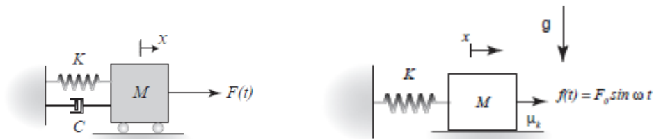
Figure 5.14 a) Diagram of cable damping concept; b) Diagram of cable with damper. Reproduced from: Guy Cable Design and Damping for Vertical Axis Wind Turbines: Sandia National Laboratories, energy report.
