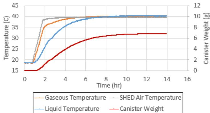
Figure A.4: Temperatures and canister weight with a 60 % liquid volume with the jerrycan lying down using LEVIII fuel.
