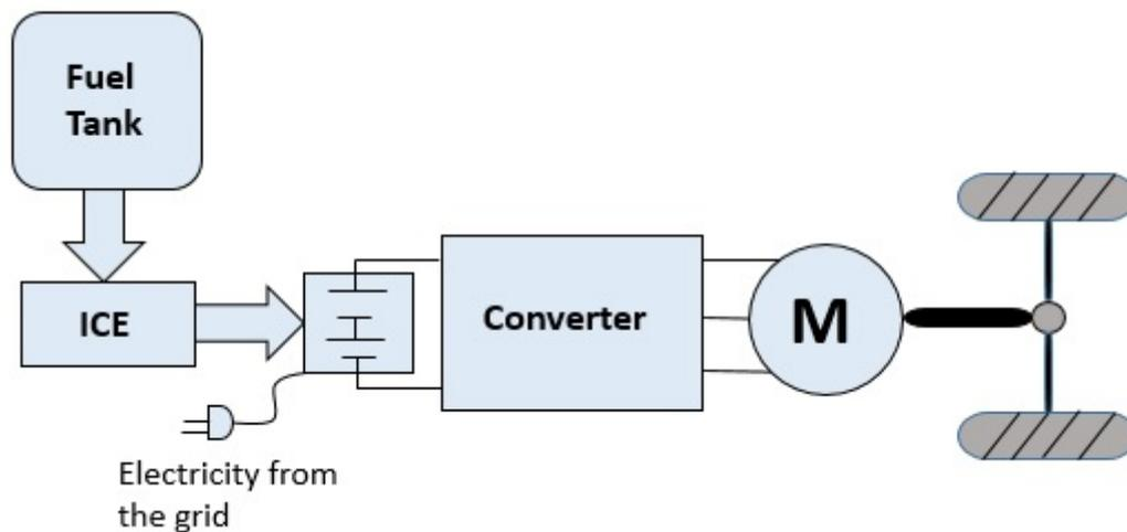
Figure 1.1: Schematic picture of a PHEV powertrain, where M is the electrical motor and ICE the internal combustion engine.
