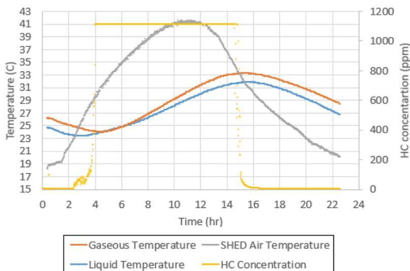
Figure 5.15: Temperatures and FID signal to detect the hydrocarbons evaporating from the fuel tank.
