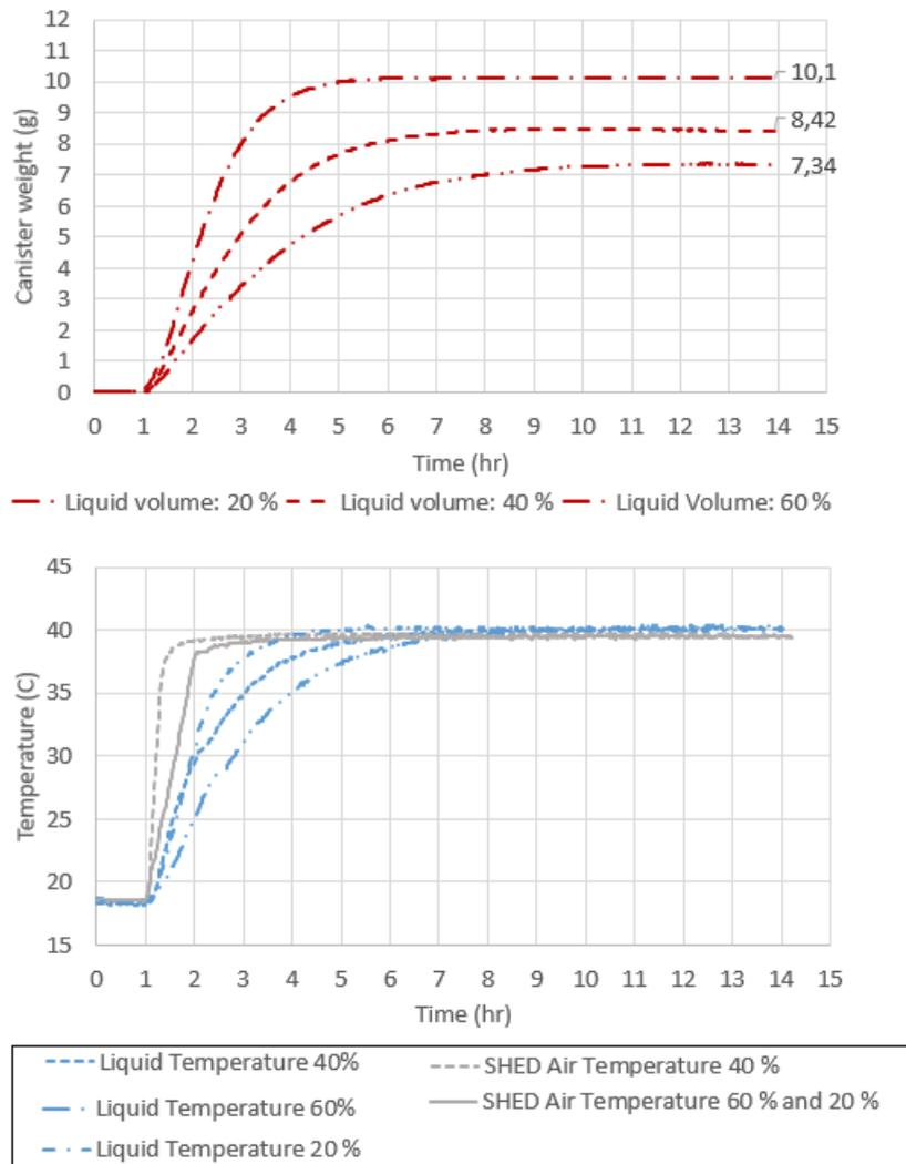
Figure 5.7: Continuously measured canister weights and temperatures from experiments with LEVIII fuel exposed to a temperature step. The liquid volume was equal to 4, 8 and 12 litres of gasoline.
