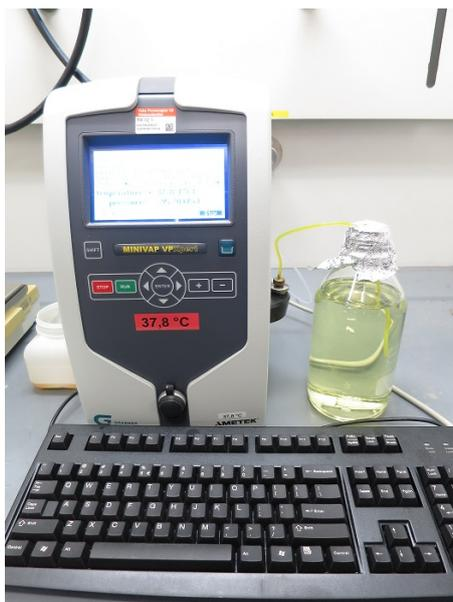
Figure 4.1: The vapor pressure gauge to the left performing a vapor pressure test of the gasoline in the glass bottle to the right.
