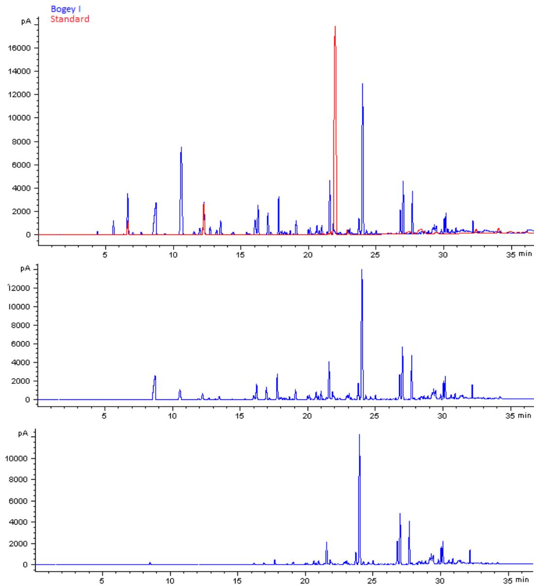
Figure A.1: BogeyI gasoline composition initially and after 16 and 47 mass% had been evaporated.
