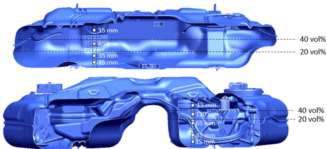
Figure 4.7: A schematic picture of the placement of the thermocouples in the fuel tanks.
