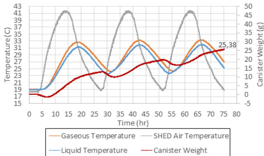
Figure 5.14: Resulting temperatures and canister weight from three consecutive CARB cycles with the fuel tank on-board a vehicle. LEVIII gasoline was used, and the scale and canister were placed inside the SHED.
