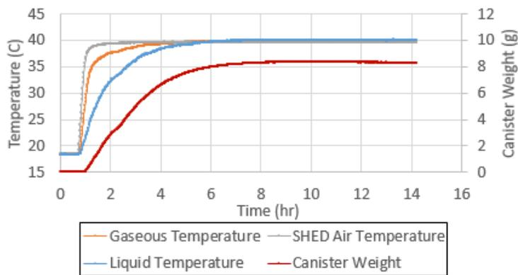
Figure A.3: Temperatures and canister weight with a 40 % liquid volume with the jerrycan lying down using LEVIII fuel.
