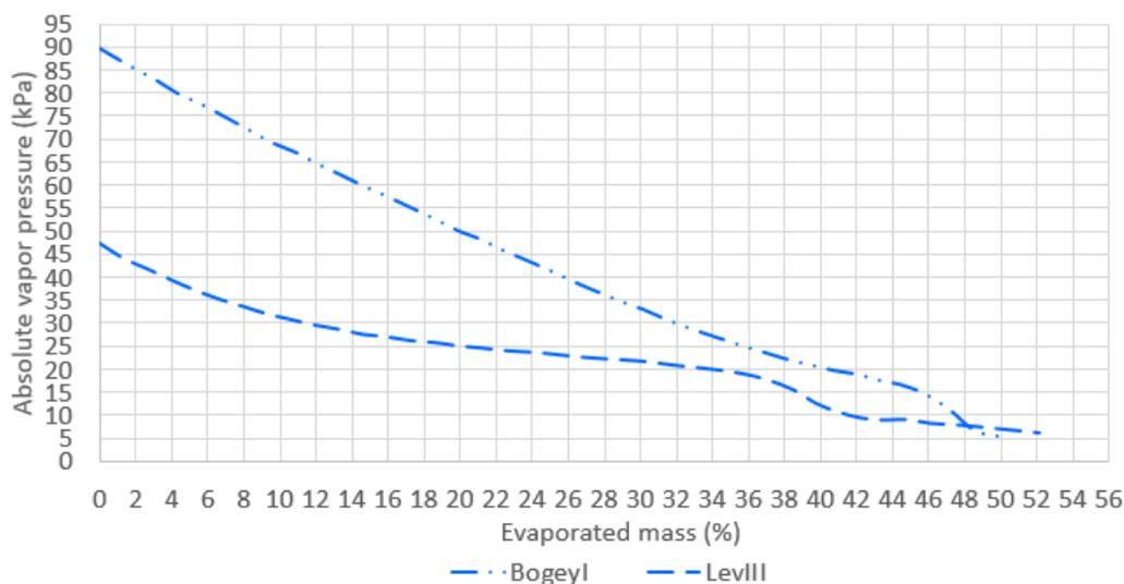
Figure 5.1: The evaporation curve for BogeyI and LEVIII.
