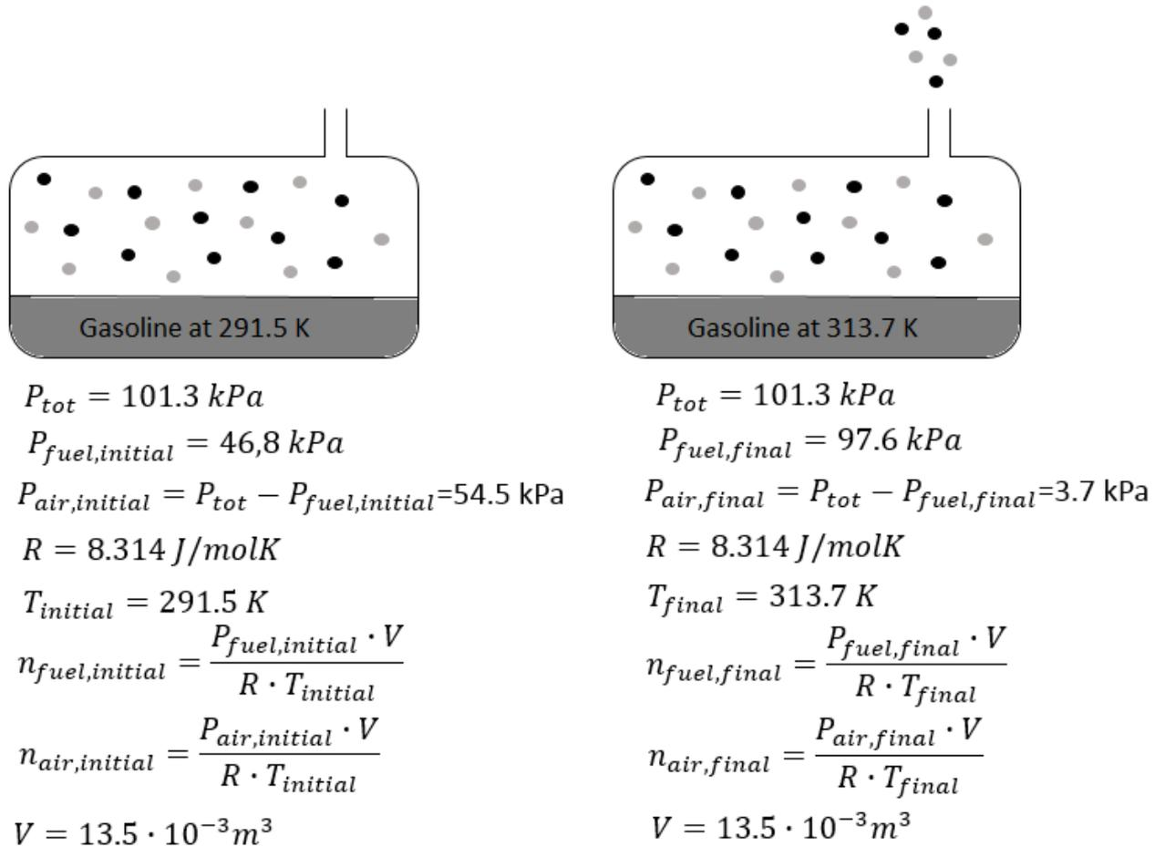
Figure B.1: A schematic setup over the initial and final system and all the values.
