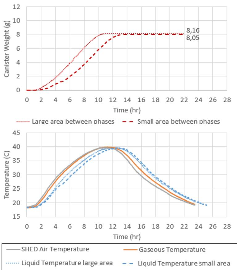
Figure 5.9: Continuously measured canister weights and temperatures from experiments with LEVIII fuel exposed to a CARB temperature cycle.
