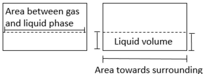
Figure 4.5: Schematic picture of the definitions of area and area-to-volume ratio.
