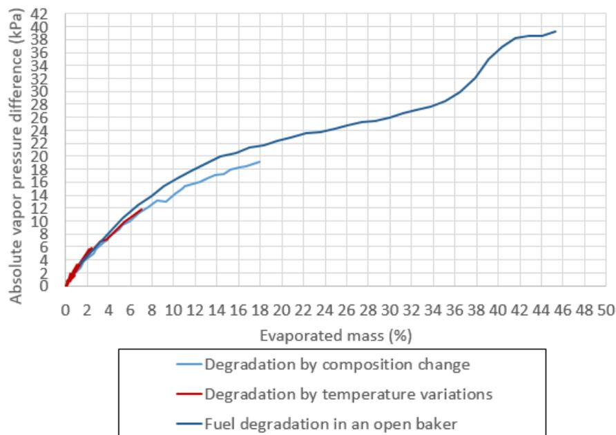
Figure 5.17: Absolute vapor pressure change as a function of evaporated mass for LEVIII.
