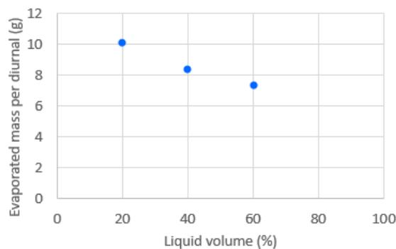
Figure 5.8: Expelled mass as a function of liquid volume with the jerrycan lying down. A smaller liquid volume results in a larger gaseous volume and more hydrocarbons evaporate.
