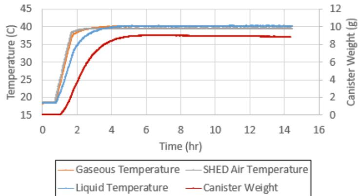
Figure A.2: Temperatures and canister weight with a 20 % liquid volume with the jerrycan lying down using LEVIII fuel.
