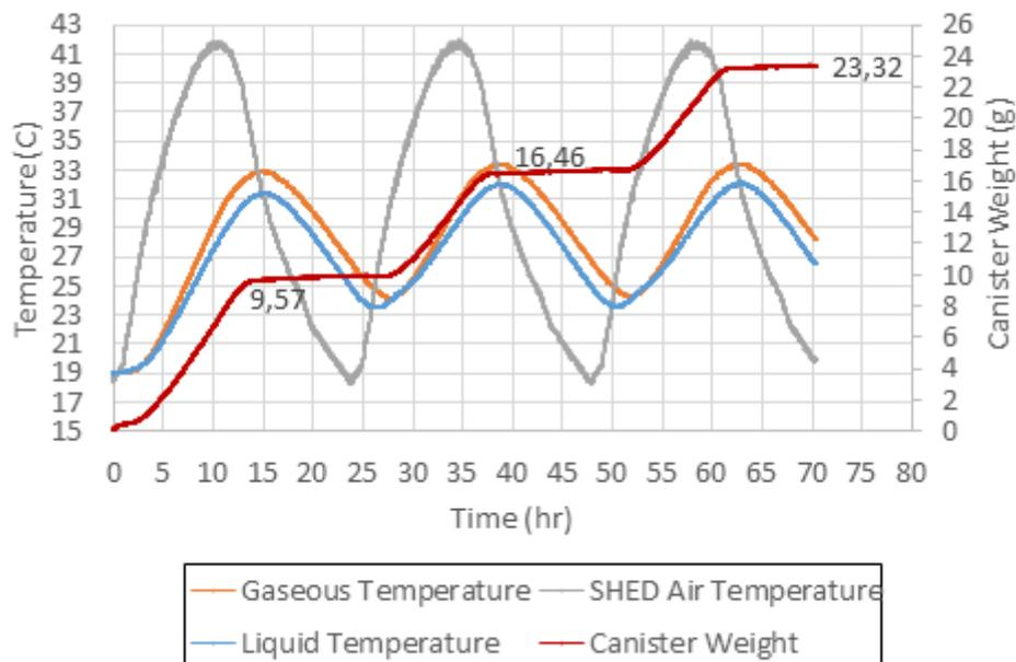
Figure 5.16: Resulting temperatures and canister weight from three consecutive CARB cycles with the fuel tank on-board a vehicle. LEVIII gasoline was used, and the scale and canister were placed outside the SHED.
