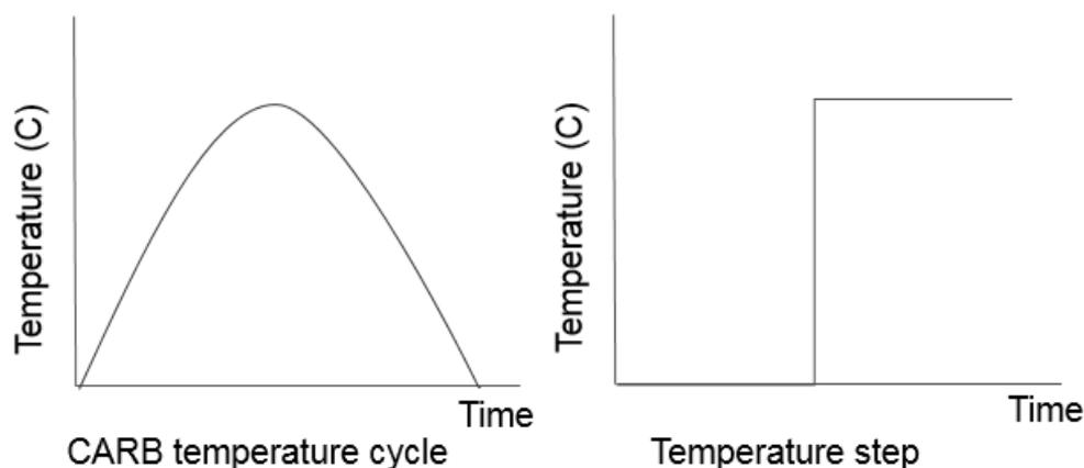
Figure 4.3: Schematic picture of a CARB temperature cycle and a temperature step. The minimum and maximum temperatures are equal to  $18.33\text{ }^{\circ}\text{C}$  and  $40.55\text{ }^{\circ}\text{C}$ .
