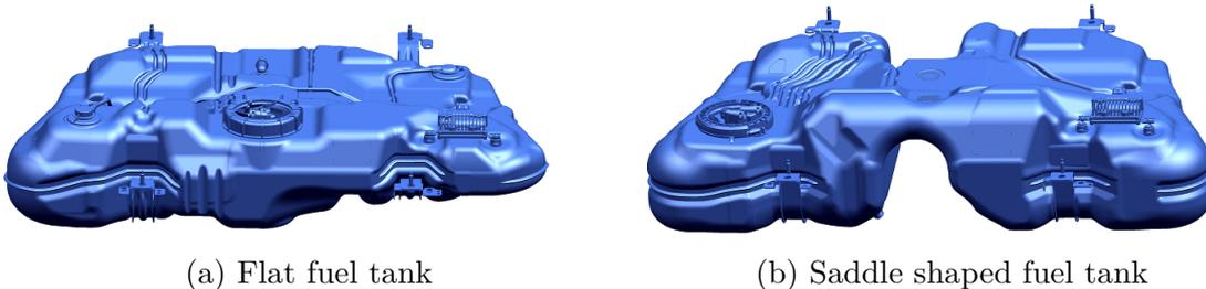
Figure 2.3: Geometry difference between fuel tanks.
