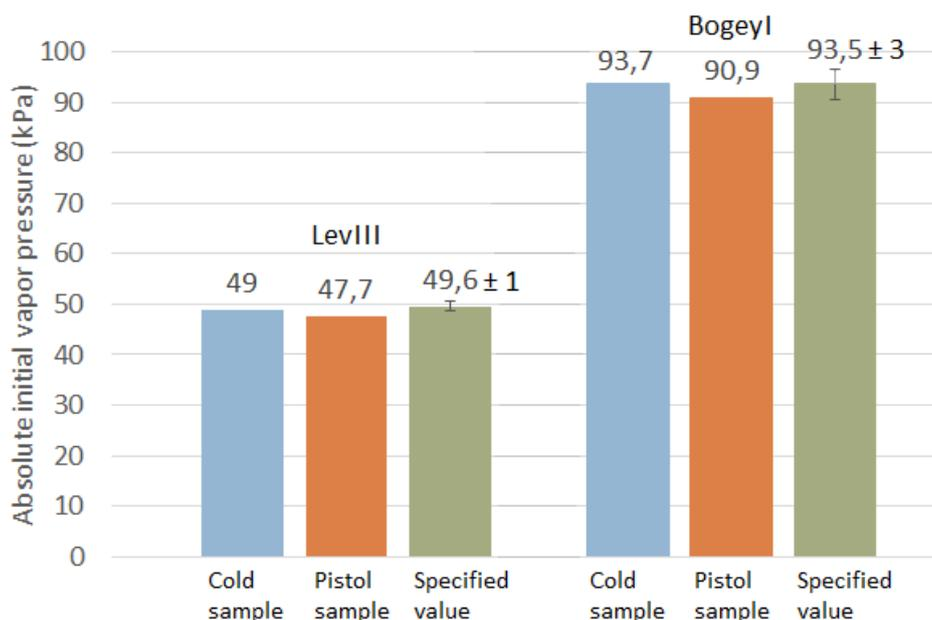
Figure 5.3: Measured vapor pressure with the two different sampling methods and the specified acceptable range.
