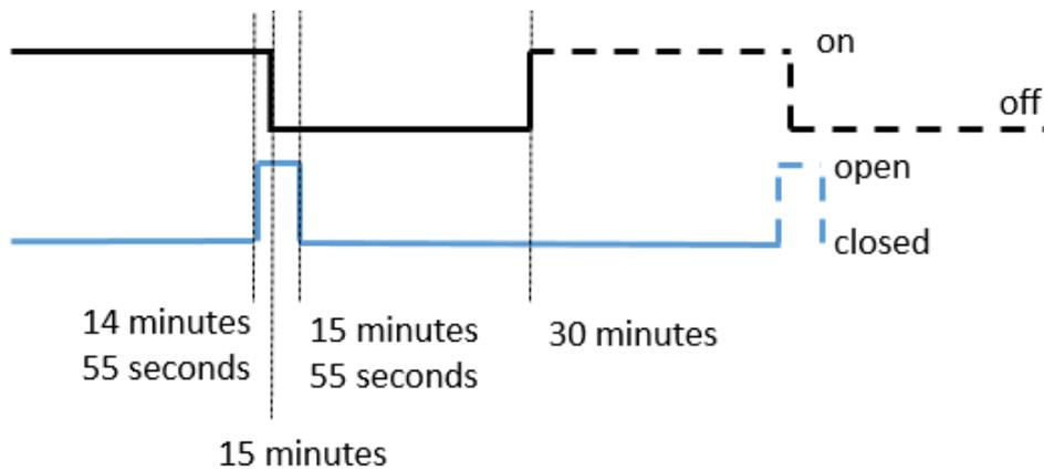
Figure 4.10: The control-scheme used to program the PLC. The upper line represent the vacuum pump and the lower line the valve used to add fresh air to the fuel tank.
