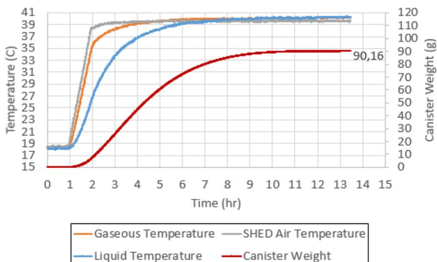
Figure 5.11: Temperatures and canister weight from the experiment using BogeyI gasoline. The large amount of expelled hydrocarbons is due to that the gasoline is boiling inside the fuel tank.
