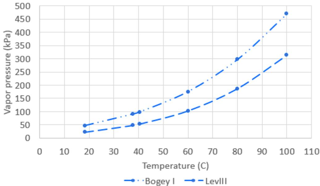
Figure 5.4: Vapor pressure curves describing the vapor pressure as a function of temperature for LEVIII and BogeyI.
