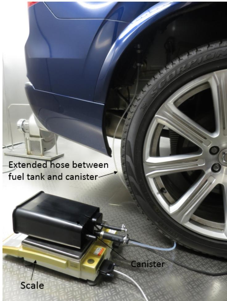
Figure 4.8: The car canister is located by the right rear wheel. An extended hose was added to be able to place an external canister on a scale.
