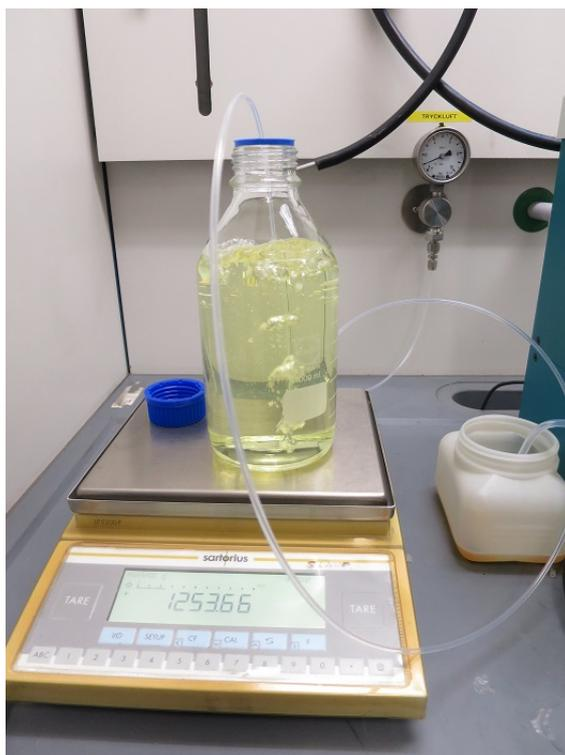
Figure 4.2: Gasoline is boiled off by bubbling compressed air through it.
