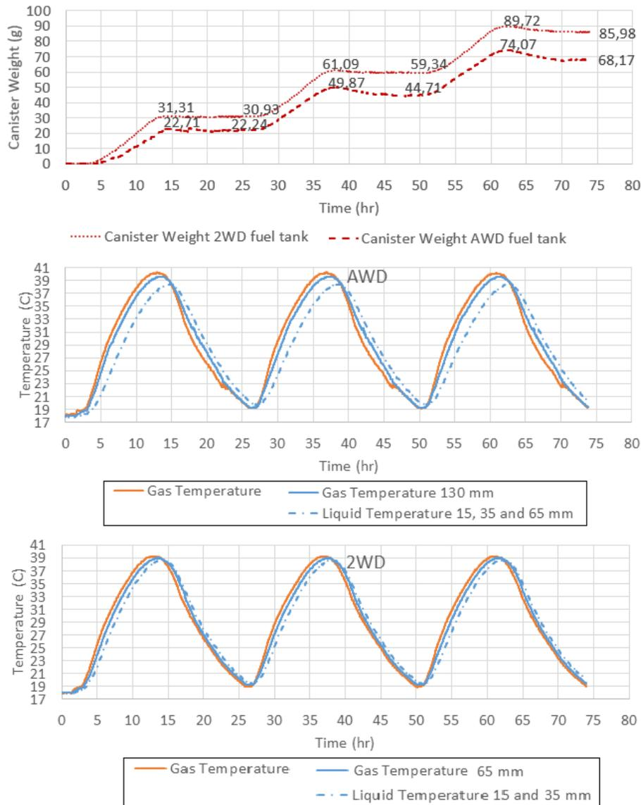
Figure 5.13: Resulting canister weights and temperatures from experiments with an AWD and 2WD fuel tank filled to 20 vol% with LEVIII gasoline.
