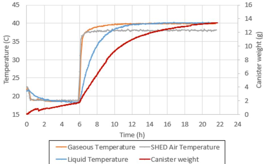
Figure 5.5: Continuously measured temperatures and canister weight with LEVIII fuel and ambient air used as carrier gas. After 6 hours the temperature was raised from 18.33 °C to 40.55 °C.
