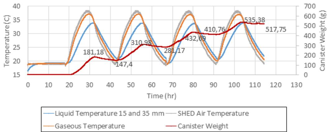
Figure A.5: Temperatures and canister weight with a 40 % liquid volume with the 2WD fuel tank using BogeyI gasoline.
