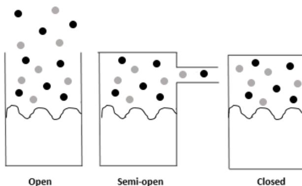
Figure 2.5: Schematic picture of open, semi-open and closed systems.
