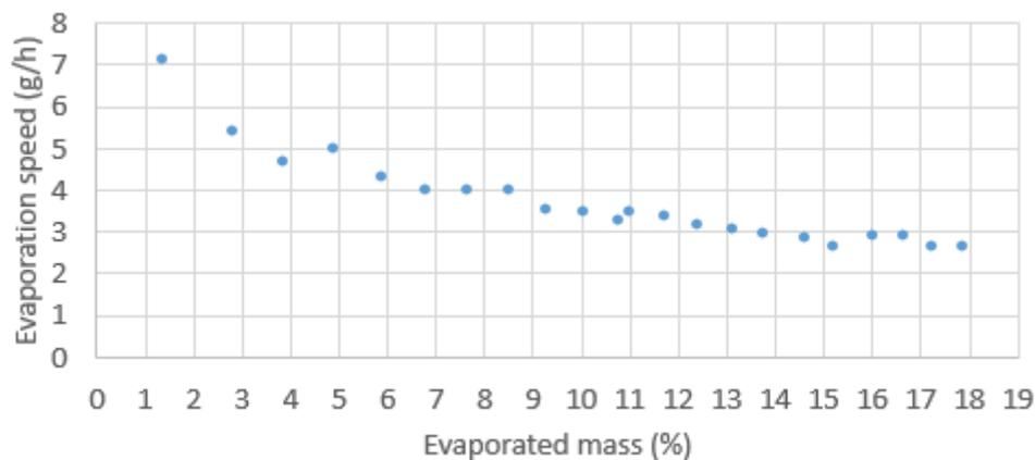
Figure 5.18: Evaporation rate as a function of evaporated mass with the vacuum pump system. As shown the evaporation rate is lowered as hydrocarbons boil off and the vapor pressure is reduced.
