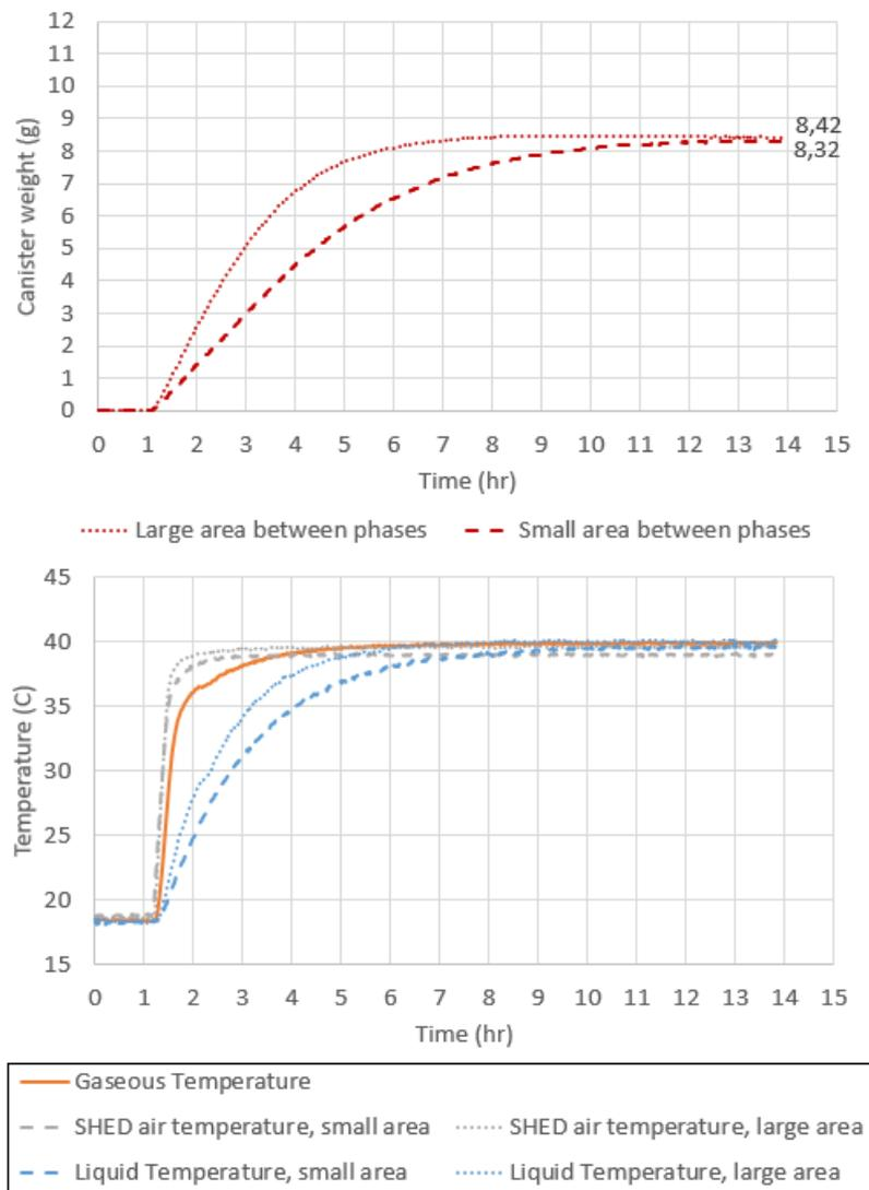
Figure 5.6: Continuously measured canister weights and temperatures from experiments with LEVIII fuel exposed to a temperature step. The jerrycan was placed laying down and standing up to generate a large respectively small area between liquid and gaseous phase.
