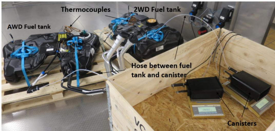
Figure 4.6: The experimental setup used to perform the experiments with fuel tanks.
