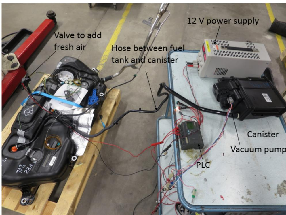
Figure 4.9: The experimental setup used to speed up the evaporation process to study the fuel degradation over an extended time.
