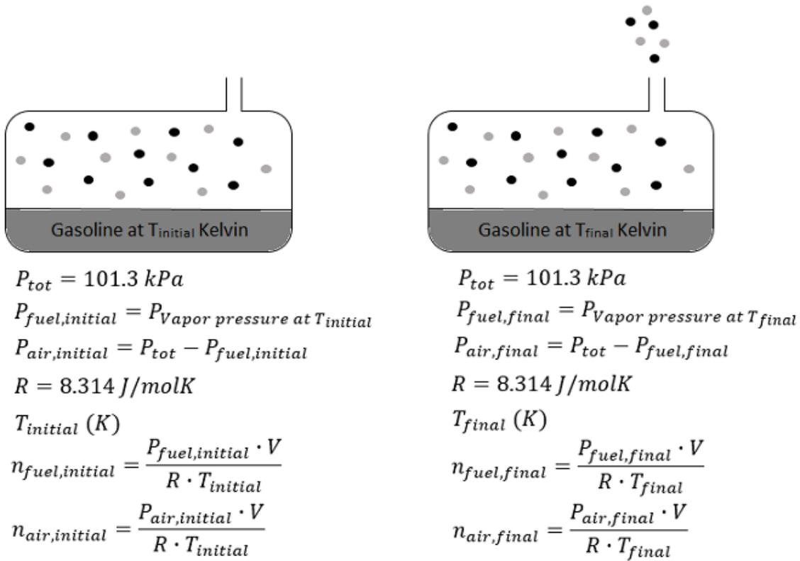
Figure 2.6: Effects of a temperature increase in a vented fuel tank.
