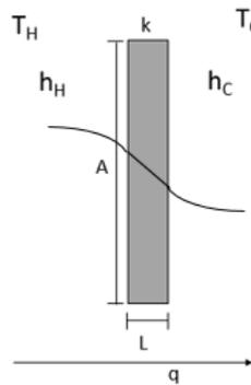
Figure 2.7: Schematic picture of the heat transport from a hot fluid to a cold fluid through a wall of thickness  $L$ .
