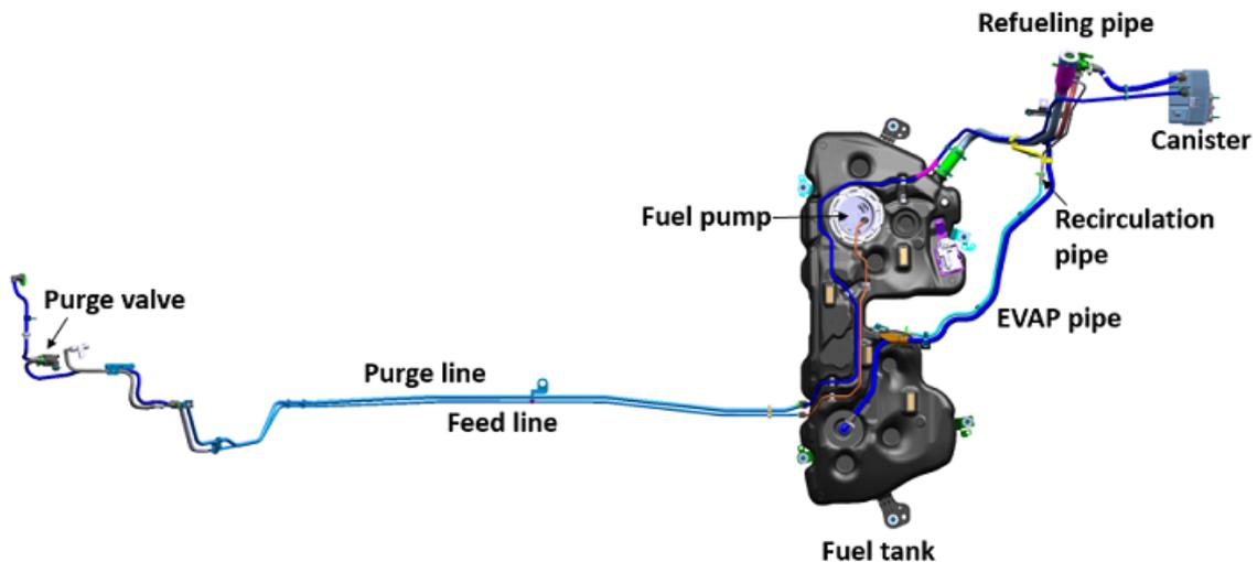
Figure 2.1: An overview of the gasoline fuel system.
