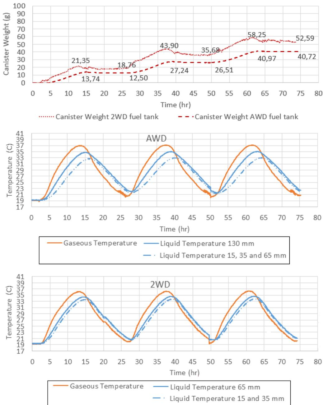
Figure 5.12: Resulting canister weights and temperatures from the experiments with an AWD and 2WD fuel tank filled to 40 vol% with LEVIII gasoline. The strange drop at the end of the second cycle in the bottom curve is due to a canister swap.
