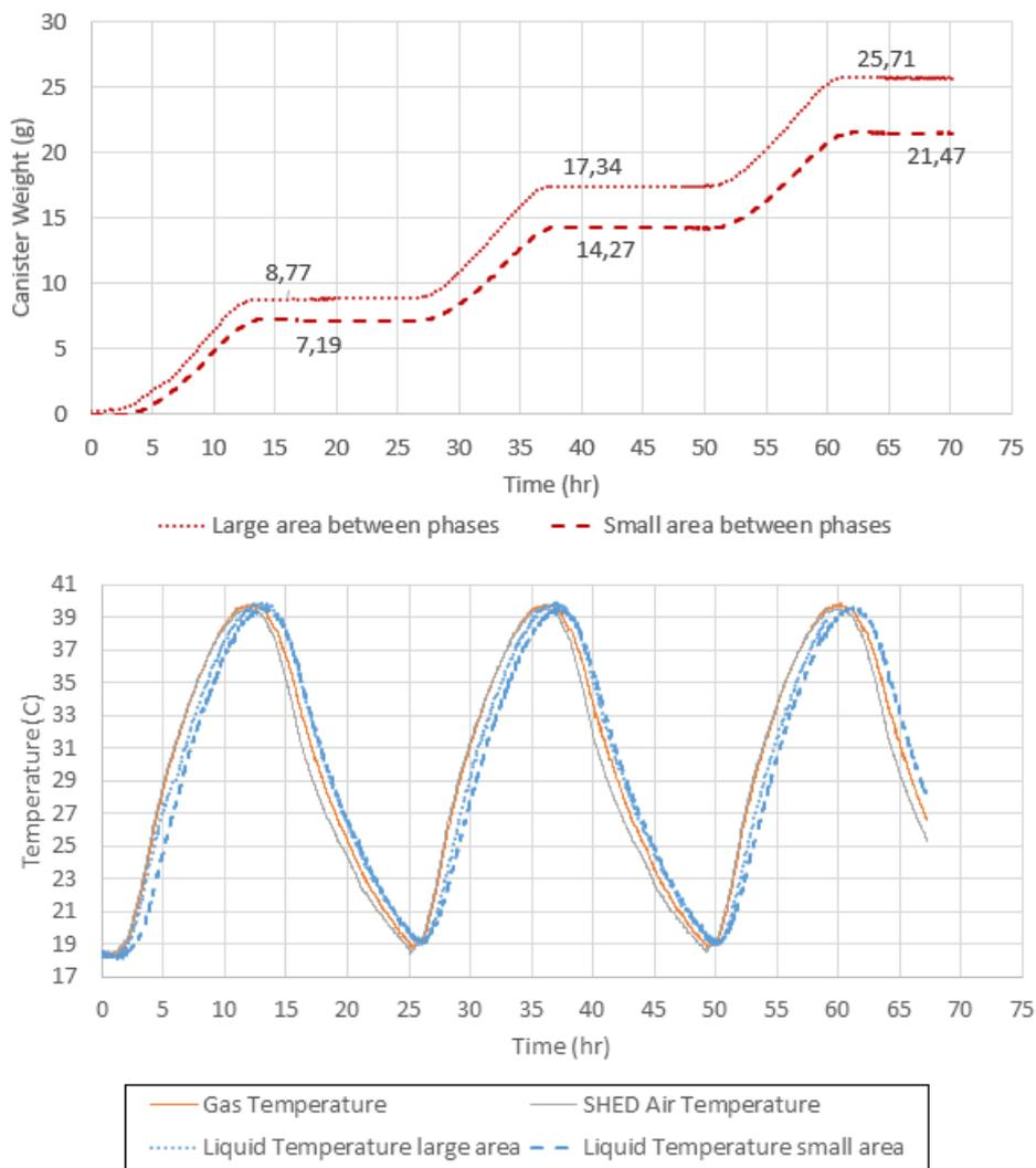
Figure 5.10: Continuously measured canister weights and temperatures from experiments with LEVIII fuel exposed to 3 consecutive CARB temperature cycles.
