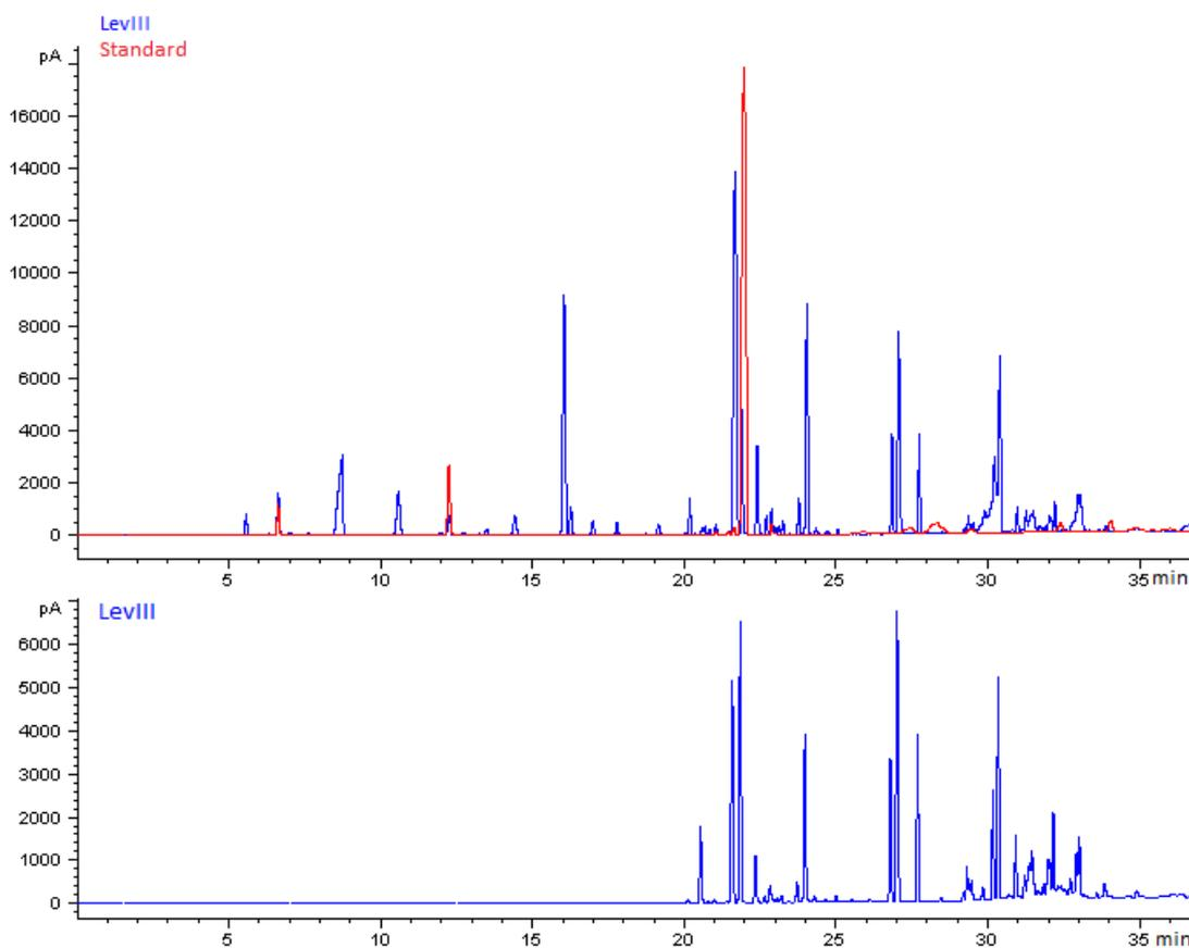
Figure 5.2: LEVIII gasoline composition, initially and after 51 mass% had been evaporated.
