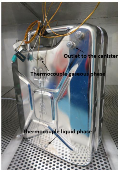
Figure 4.4: The stainless steel jerry can that was used in the experiments.
