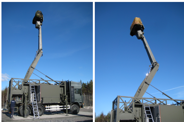
(c) Attachment of camouflage net 101362 during visibility tests on GIRAFFE AMB. (d) Attachment of camouflage net 101593 during radar performance tests on GIRAFFE AMB.
