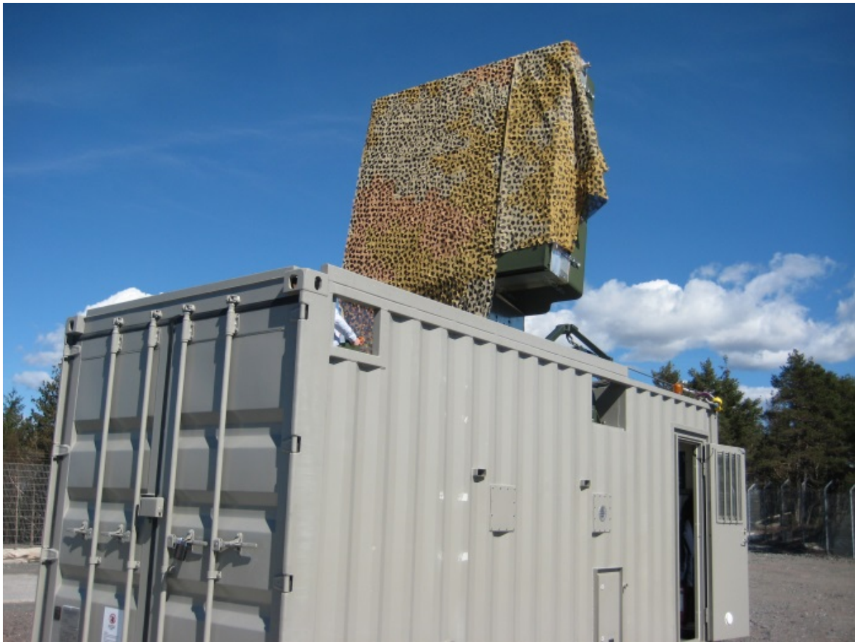
Figure 3.7: Attachment of camouflage net 101593 on the GIRAFFE 4A antenna.
