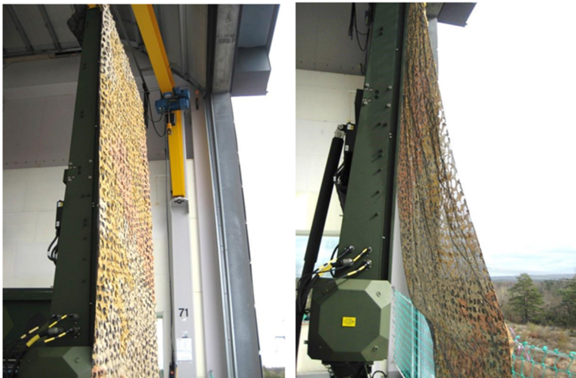
(a) Attachment of camouflage net 101593 on the ARTHUR antenna in straight position. (b) Attachment of camouflage net 101593 on the ARTHUR antenna in tilted position.
