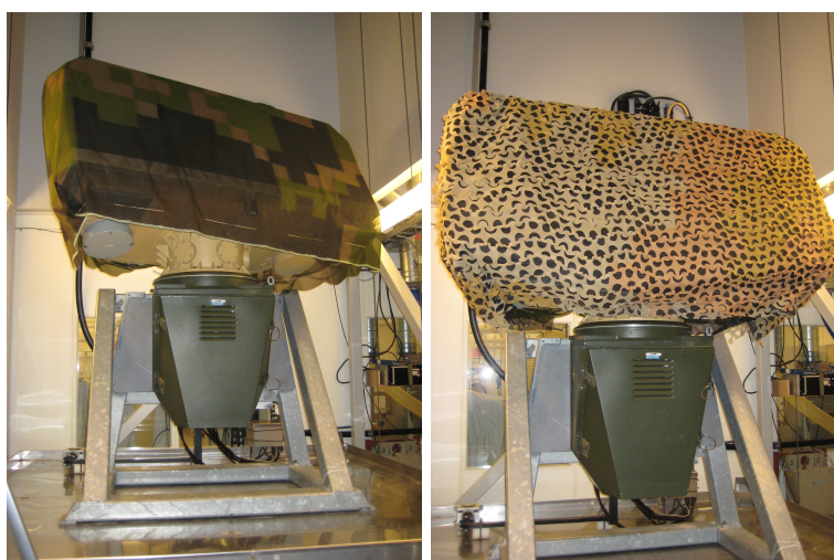
(a) Attachment of camouflage net 101362 during radar performance tests on GIRAFFE AMB. (b) Attachment of camouflage net 101593 during radar performance tests on GIRAFFE AMB.
