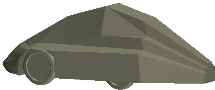
Figure 5.14: Geometry of the edgy boat tail, C_D = 0.168 .
