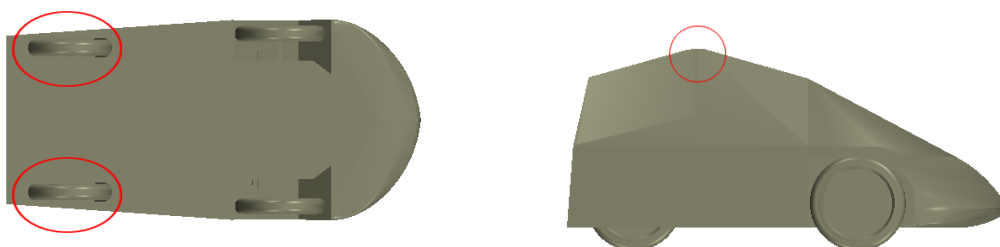
(a) Reduced wheels opening in the undercarriage around the rear wheels. (b) Rounded top.
