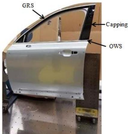
Figure 14. Components assembled on the left front door
