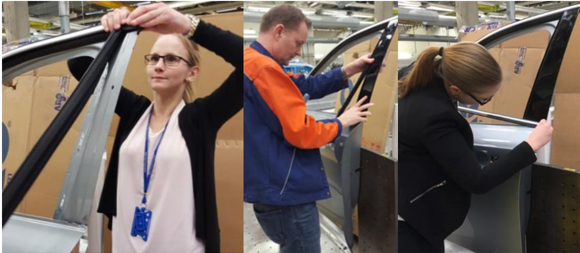
Figure 35. Mounting of GRS, OWS and capping by three assemblers
