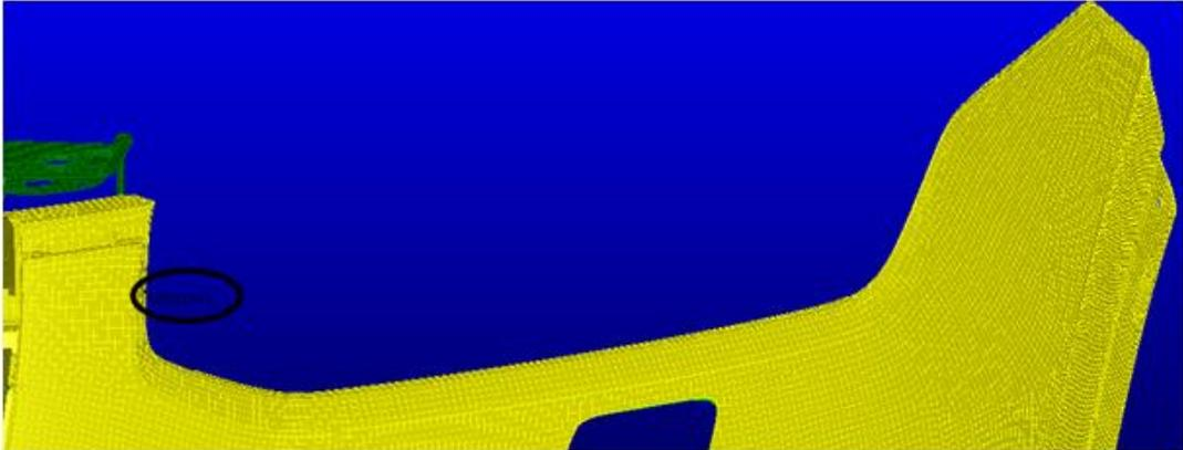
Figure 90. Measurement point located on the right side on the front bumper
