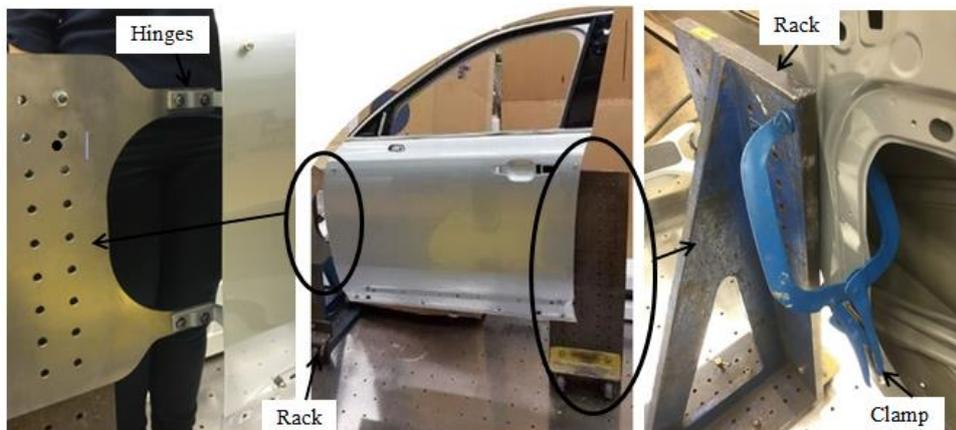
Figure 36. Positioning of the left front door in a fixture
