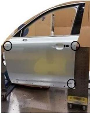
*Figure 37. Positioning of spheres on the left front door*
