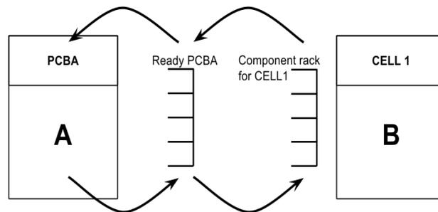
**Figure 35: Kanban between the PCBA process and the cell**
