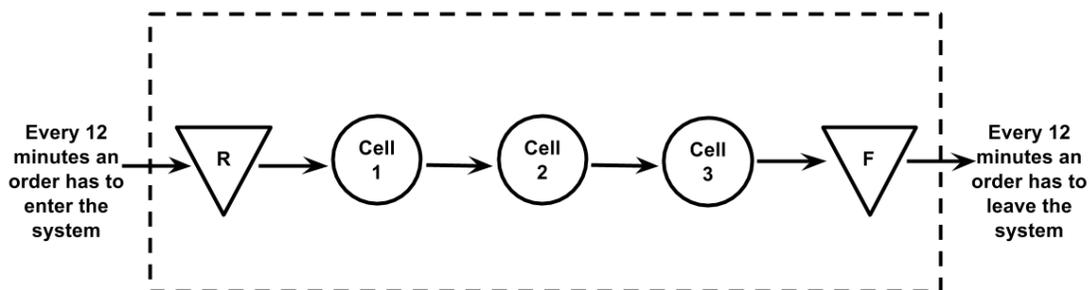
Figure 36: Generalized takt time control for the cell
