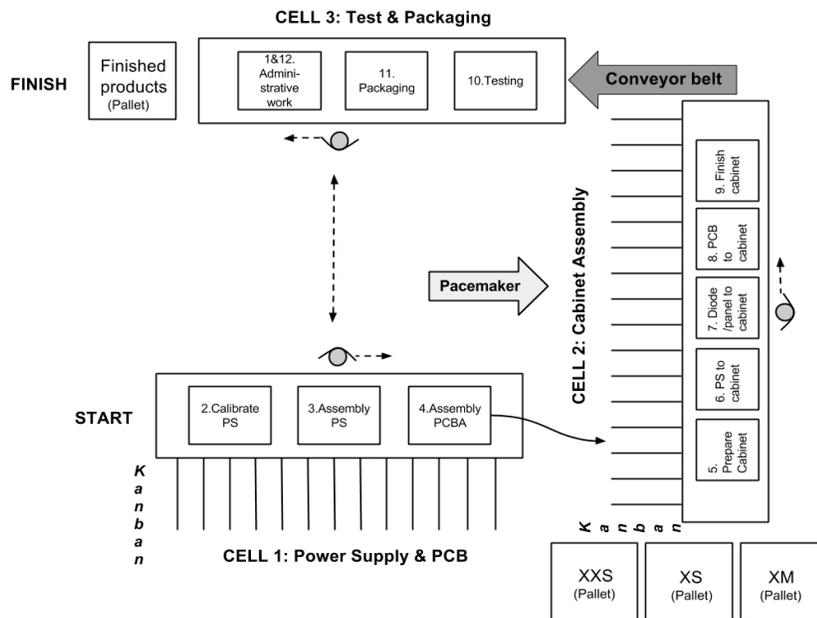
**Figure 31: Scenario three, two operators inside and one outside the U-layout**
