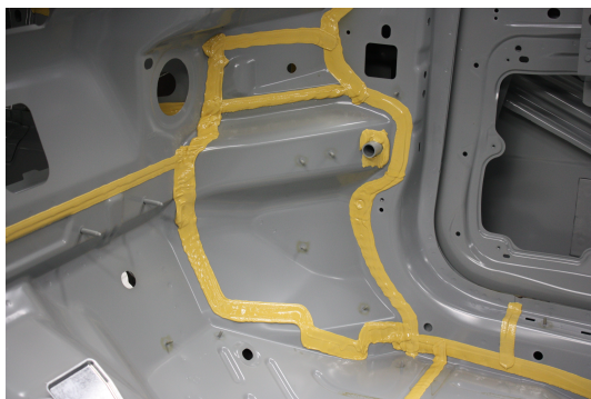
Figure 1: Flat bead sealing seams on a body-in-white.
