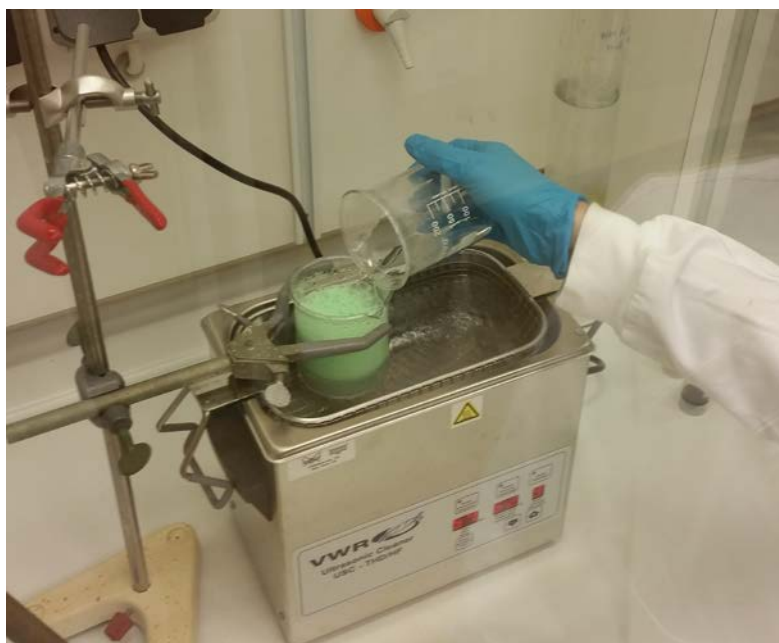
Figure 2. The producing of nanoparticles with ultrasonic water bath
