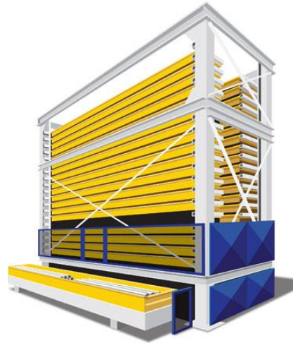
Figure 2.9 Vertical Lift Module with two rows of storage trays, one shaft in the middle and one picking area in the front (Picture of Vertical Lift Module, 2016).
