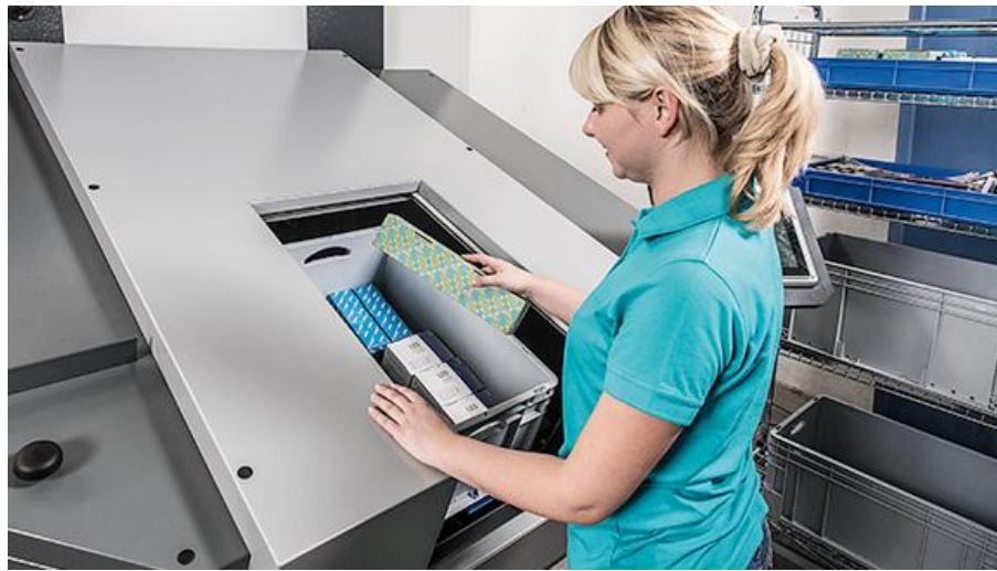
Figure 5.7 The picking station of a Kardex Remstar LR 35 (Picture of picking station at Kardex Remstar LR35, 2016).
