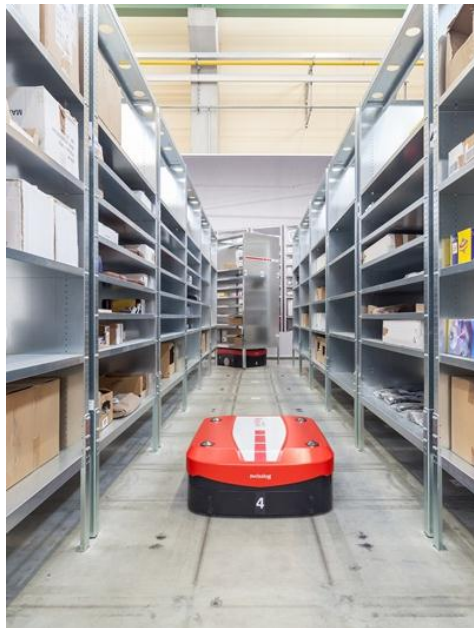
Figure 5.10 A Swisslog CarryPick AGV travelling in an aisle with another CarryPick AGV retrieving a mobile storage racks (CarryPick Storage System, 2016).
