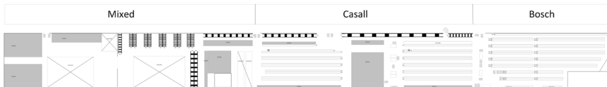
Figure 4.1 Layout of the mezzanine at KN. The area to the right is dedicated to Bosch and the area adjacent is dedicated to Casall. The area to the left of the mezzanine is a mixed zone. The white rectangles represent standard racks, the black and white striped areas represents pallet racks and the grey area are buffer zones. The crossed out white zones in the left are used for Samsung and Ericsson and disregarded in this report. The holes in the wall with pallets in front represent pallet lifts. This figure can be seen in a larger version in Appendix II.
