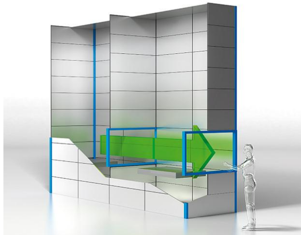
Figure 5.4 Operation principle behind the Shuttle XPmultiple (Picture of working principle behind Kardex Remstar XPmultiple, 2016).
