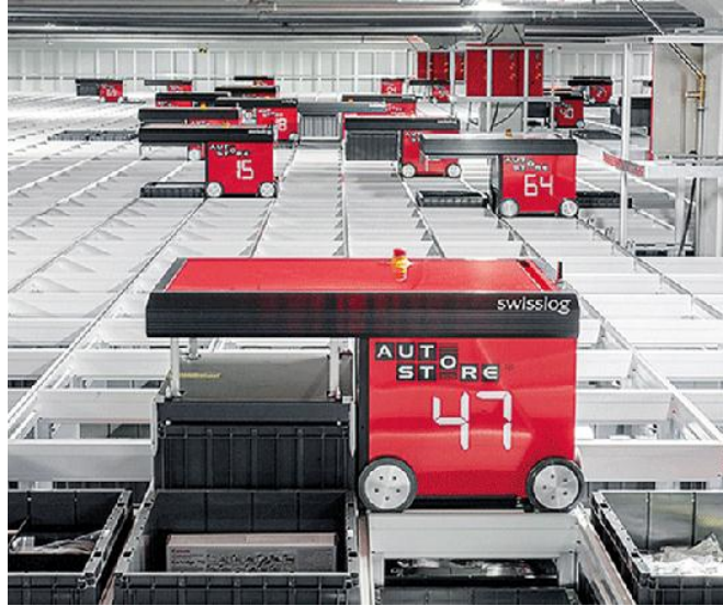
Figure 5.9 AutoRobots running on top of the AutoStore grid construction (Efficient small parts storage with AutoStore, 2016).
