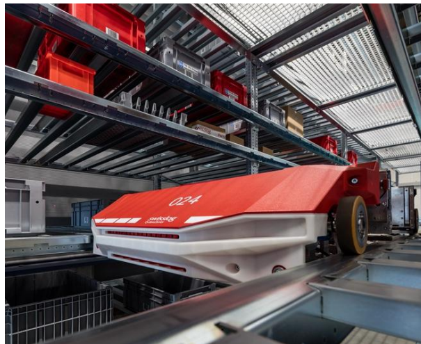
Figure 5.8 A shuttle moving in an aisle to retrieve goods (Swisslog Cyclone Carrier, 2016).
