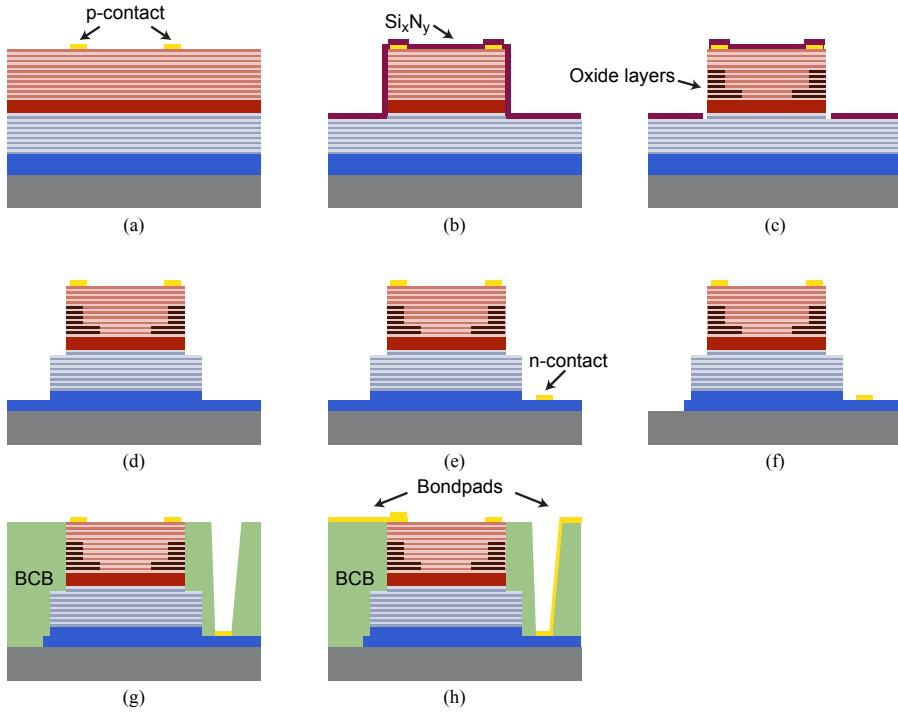
Fig. 6.2. The process steps for high-speed VCSEL fabrication includes: (a) *p*-contact deposition, (b) mesa etching followed by deposition of  $\text{Si}_x\text{N}_y$ , (c) oxide aperture formation after opening of the  $\text{Si}_x\text{N}_y$  on the mesa side walls, (d) second mesa etching, (e) *n*-contact deposition, (f) *n*-contact layer removal beneath the *p*-bondpad, (g) planarization with BCB, and (h) deposition of bondpads.
