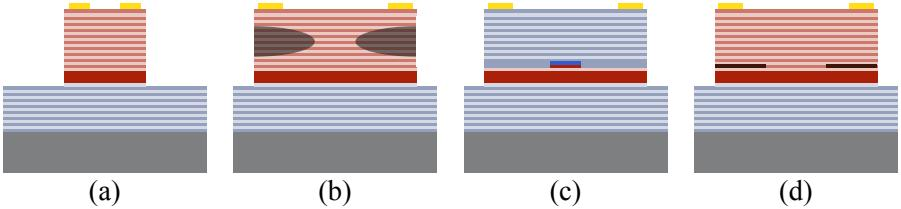
Fig. 2.2. Transverse confinement schemes: (a) etched air post, (b) ion implantation, (c) buried tunnel junction, and (d) oxide aperture.
