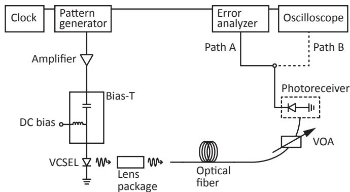
Fig. 5.2. Large signal data transmission setup. Path A is used to measure BERs, while path B is used to record eye diagrams.
