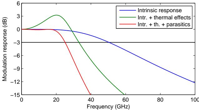
Fig. 4.1. Intrinsic and extrinsic modulation response extracted from the VCSEL used in Paper A with  $K$ - and  $D$ -factors of  $0.17\text{ ns}$  and  $9.0\text{ GHz/mA}^{1/2}$ , respectively, along with a parasitic pole,  $f_p \approx 17\text{ GHz}$ .
