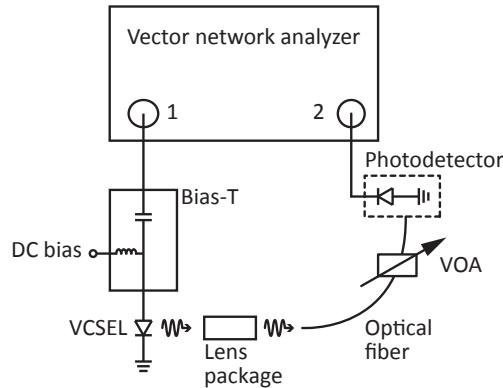
Fig. 5.1. Measurement setup for the small signal modulation response.
