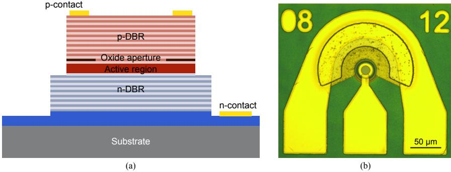
Fig. 2.1. (a) Schematic cross-section of a VCSEL, and (b) microscope top view of a VCSEL on chip.
