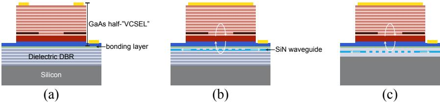
Fig. 3.1. Hybrid vertical-cavity lasers with surface emission (a), in-plane waveguide emission using a weak diffraction grating (b), and using a HCG (c).
