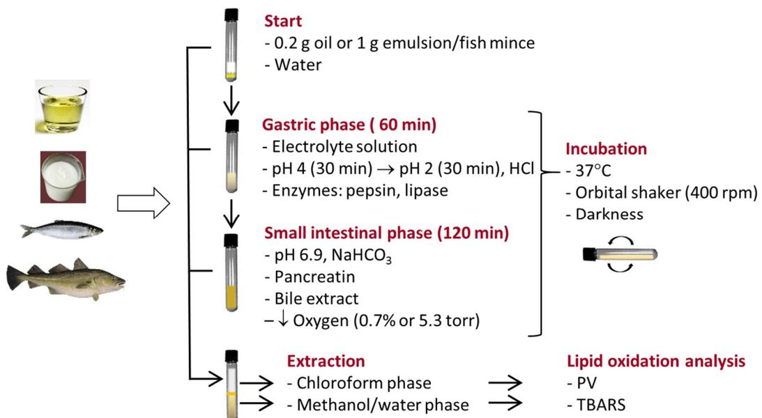
**Figure 9** Schematic overview of the static two-step digestion method simulating the gastric and the intestinal digestion.
