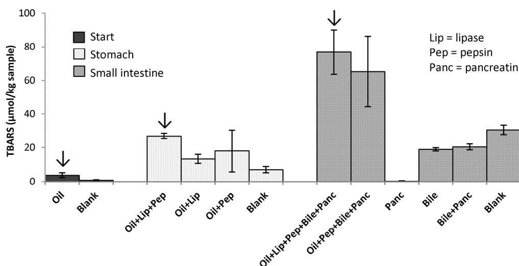
**Figure 15** Effect of digestive compounds on the formation of TBARS in cod liver oil during static digestion. The sample indicated with an arrow represents the cod liver oil subjected to the standard protocol including all digestive compounds. “Blank” is the digestion control where oil has been replaced by water. The concentration of TBARS are based on initial sample weight (oil or water). Values are mean±SD (n=3-6).
