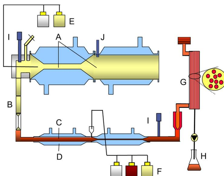
**Figure 10** Schematic overview of the tiny-TIM system: A, gastric compartment; B, pyloric sphincter; C, chyme; D, small intestinal compartment; E, gastric secretion; F, intestinal secretion; G, semi-permeable membrane (<50 nm); H, intestinal filtrate; I, pH electrodes; J, pressure sensor.
