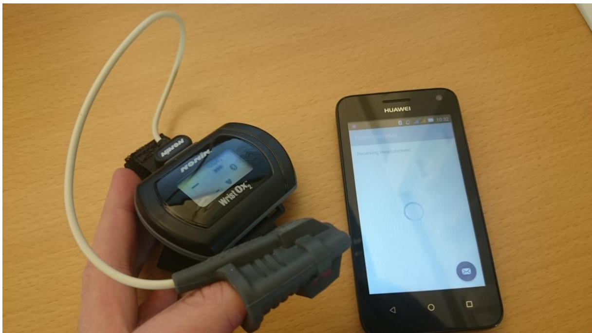
Figure 26 The gateway application receiving a measurement from a pulse oximeter
