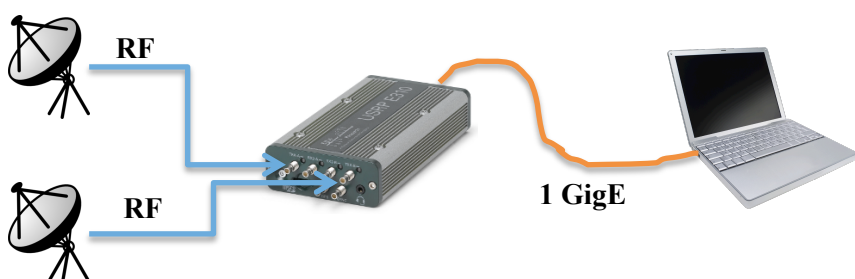
Fig. 3: Signal chain of the SALSA interferometer.
