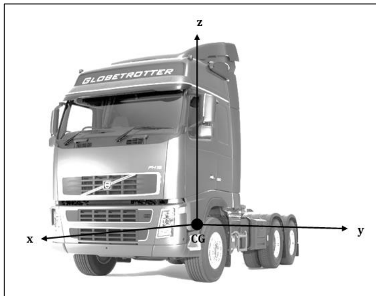
Figure 2.8 Coordinate system of a unit (tractor in this case).
