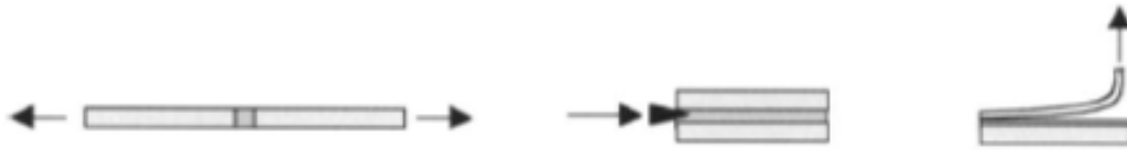
Figure 3.1 Critical loading configurations to be avoided in adhesive joint design (Left: tension; Middle: Cleavage; Right: Peel) [18]
