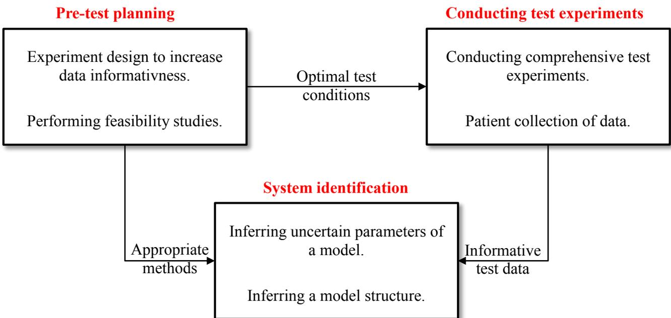
**Fig. 6:** A schematic view of the system identification process
