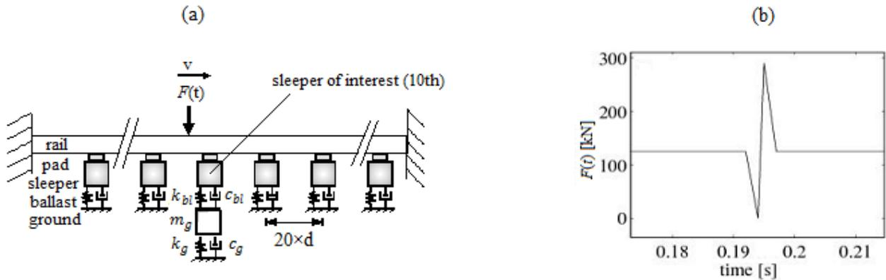
**Fig. 2.** A moving load with velocity  $v$  on a railway track with local nonlinearity or uncertainty due to the fact that sleepers put on a non-uniform ballast bed create state/parameter dependent interaction forces (a) Studied track model consisting of 20 bays of equal length. The ballast variation along the centre sleeper in bay no. 10 is of particular interest. (b) Track is subjected to a time-varying moving load  $F(t)$ . Prescribed load peaks at the passage of the center sleeper.
