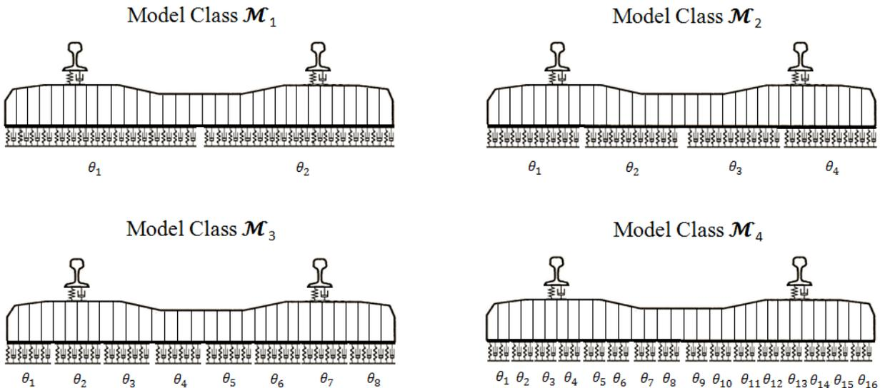
**Fig. 3.** Four candidate model classes with 2, 4, 8 and 16 free independent parameters for representing stochastic ballast bed conditions under the sleeper of interest in bay number 10. Subdivision of the sleeper indicates that the sleeper of interest is divided into 32 Euler-Bernoulli elements. Sleepers in other bays are represented by 10 Euler-Bernoulli beam elements.
