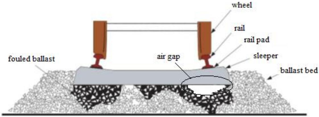
**Fig. 1.** An illustration of ballast configuration variation along a sleeper (from [14]). A significant variation of ballast density along sleeper-ballast interface may occur due to different loading conditions, poor maintenance or quality of ballast.
