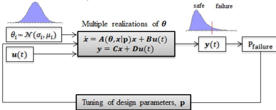
**Fig. 4:** A schematic view of the process of reliability-based design optimization of design parameter vector  $p$ . Optimization with multiple iterations to converge demands a large number of realizations of random parameter vector  $\theta$  and associated simulations to compute the failure probability  $P_{\text{failure}}$  at every major step of optimization iteration.
