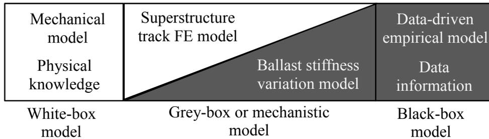
**Fig. 5:** Statistical modelling of physical systems known as grey-box modelling. This strategy has been utilized for establishing predictive models of railway track structure.
