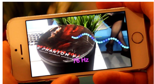
Figure 1. The Hamlin smartphone app displays a visualization on top of the Hamlin device with a fiducial marker.
