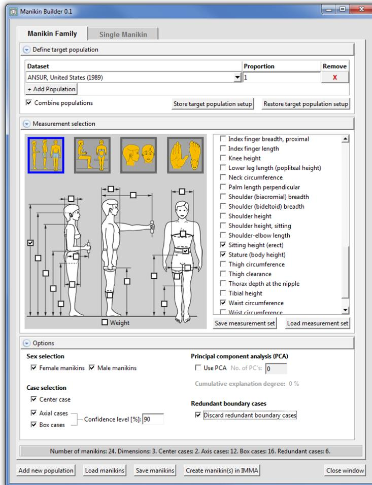
Figure 42 Interface of the anthropometric module showing the manikin family tab
