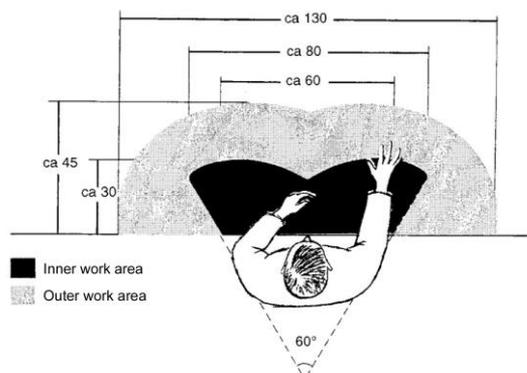
**Figure 4** Functional dimensions of horizontal arc of grasp and normal working area, measurements in centimetres (Swedish Work Environment Authority, 1998)
