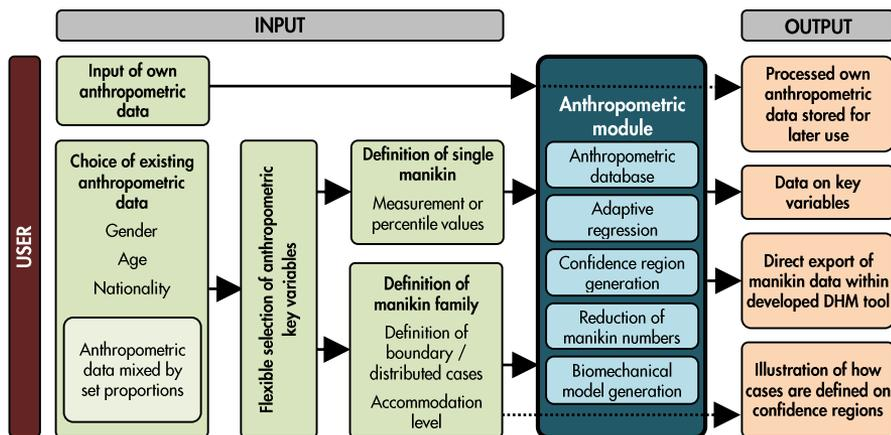
**Figure 23** Process chart illustrating the necessary parts of an anthropometric module in a DHM tool
