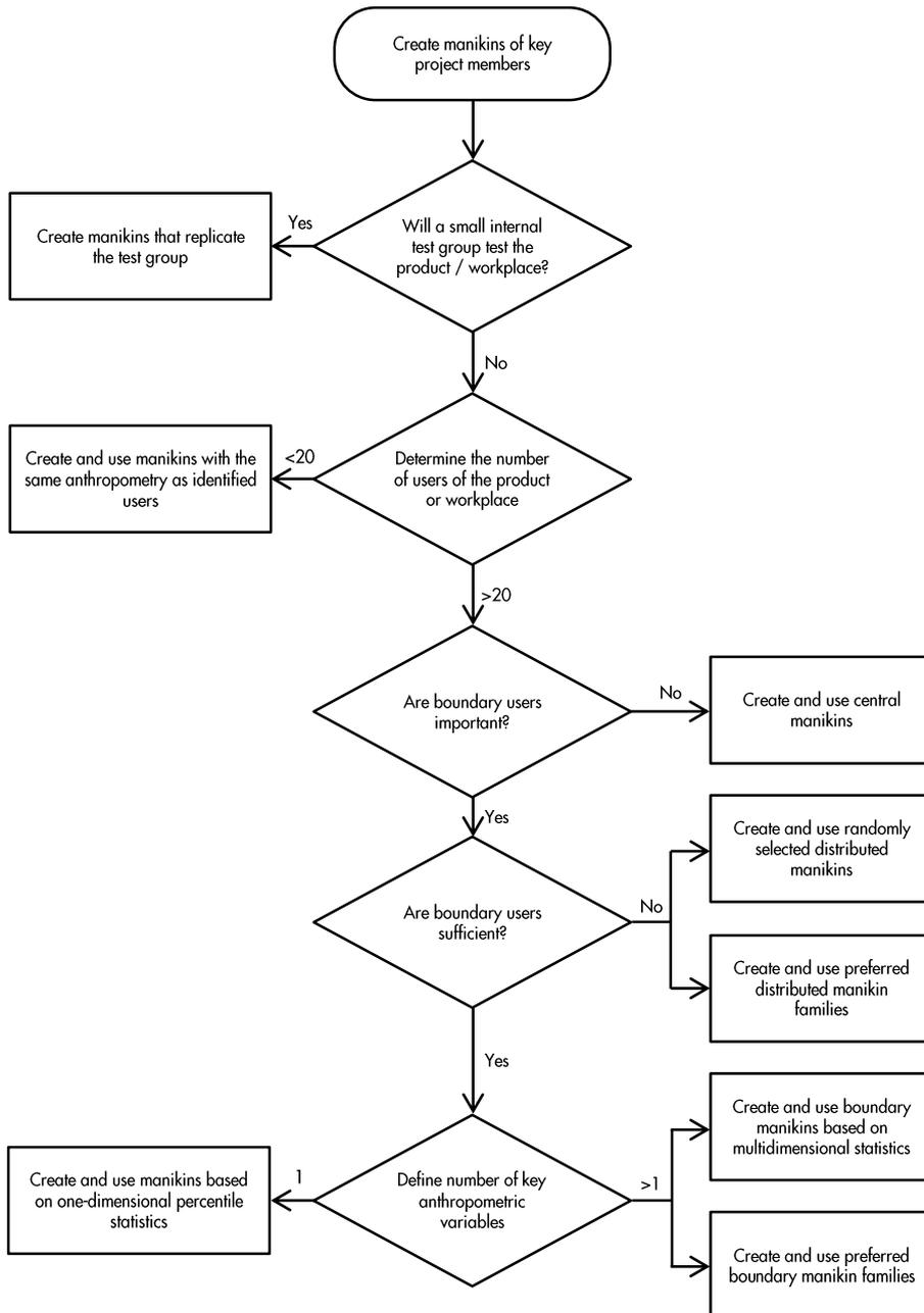
**Figure 17** Flowchart as a guide to select user representation method: replicas of identified users, central, distributed or boundary manikins (modified from Dainoff et al., 2004; Hanson and Högberg, 2012)
