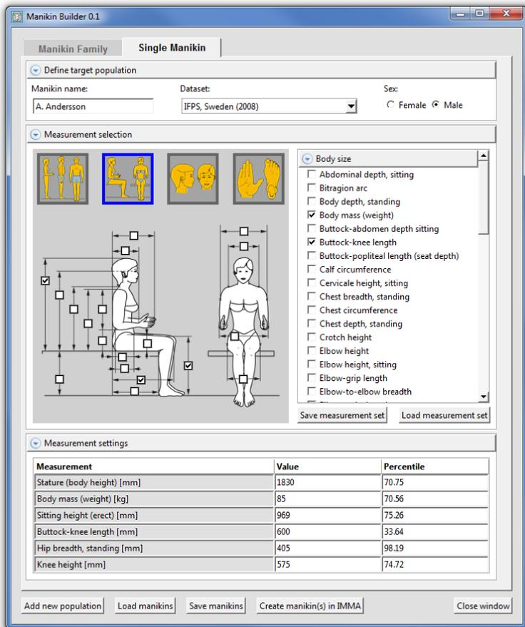
Figure 43 Interface of the anthropometric module showing the single manikin tab
