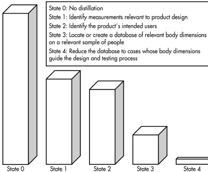
**Figure 3** The information distillation process when using anthropometric data in design, adapted from Dainoff et al. (2004)
