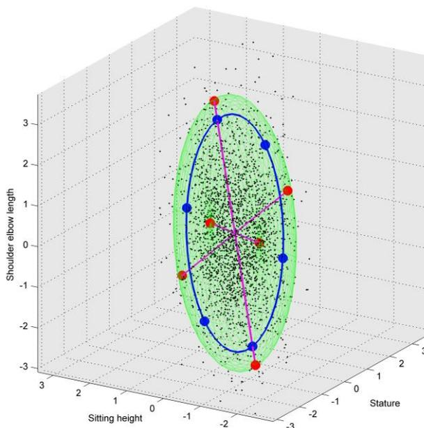
**Figure 27** A three dimensional 90% confidence ellipsoid as well as boundary cases at the axial end points of the ellipsoid and in the direction of the first and second principal component (scales in standardised z-score)
