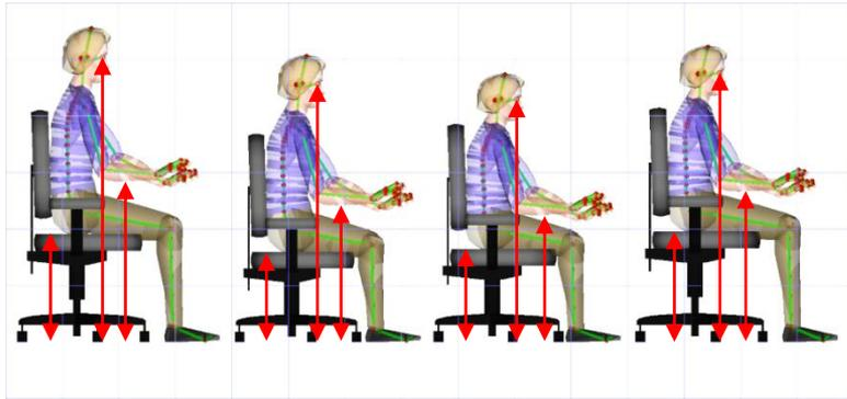
**Figure 24** Manikins in seated posture with distances measured for the design dimensions seat height, table height and eye height
