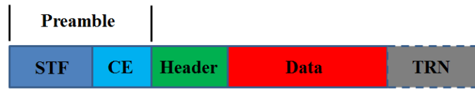
Figure 2: General structure of 802.11ad frame (source: [10])
