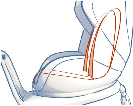
Figure 21. Mechanical advantage harness system.
