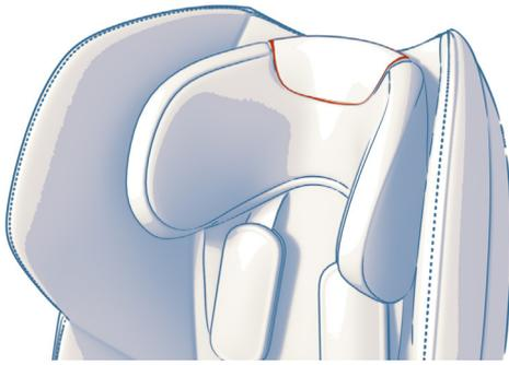
Figure 19. Headrest height adjusted by operating the lever placed in the top.
