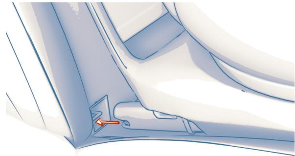
*Figure 2. ISOFIX connectors and anchor points.*
