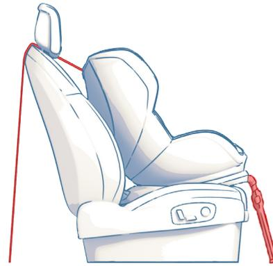
Figure 15. Top tether strap and support leg.
