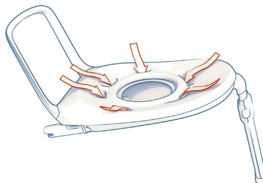
Figure 23. Ducts through the base to prevent gathering of dirt between the base and the seat.
