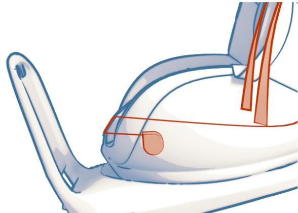
Figure 22. Spool for gathering excess tensioning belt.
