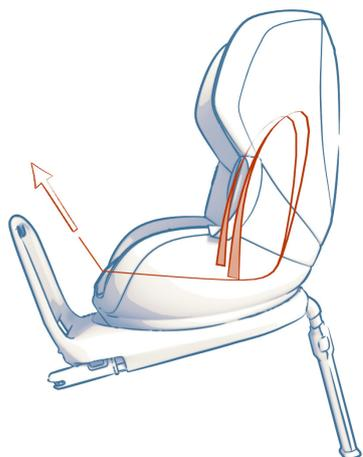
Figure 6. Force used to tighten the harness.
