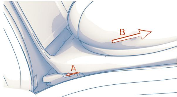
*Figure 8. The button on the ISOFIX connector is first pushed to release it from the anchor point, after which force is applied to the connector in the opposite direction.*
