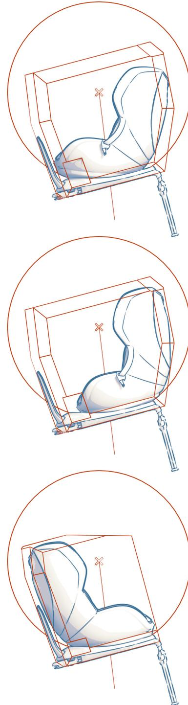
*Figure 24. Size constraints, rotation sphere and rotation axis of the seat.*
