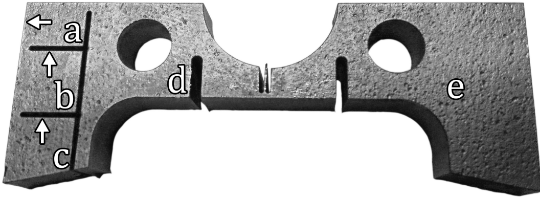
Figure 3.2: Test samples with sections cut but not separated and named according to figure, arrows indicate the side of transverse pieces facing up in mountings
