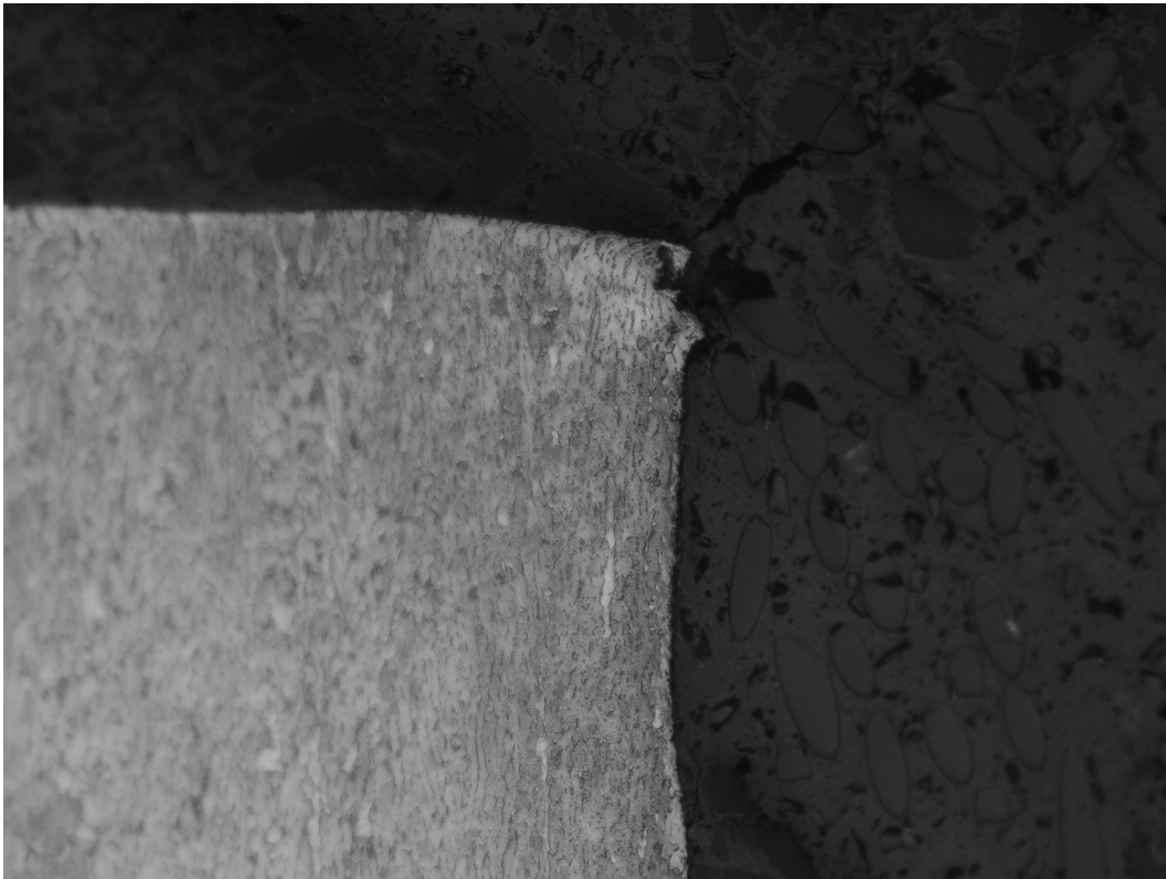
Figure 5.3: Large defect in the kerf entrance, complicating measurements of edge rounding
