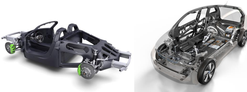
Figure 4. Left: Body structure of Porsche 918 with a CFRP main structure and metal front and rear structures [10]. Right: BMW i3 with front and rear structures in metal and the passenger cell in CFRP [11].
