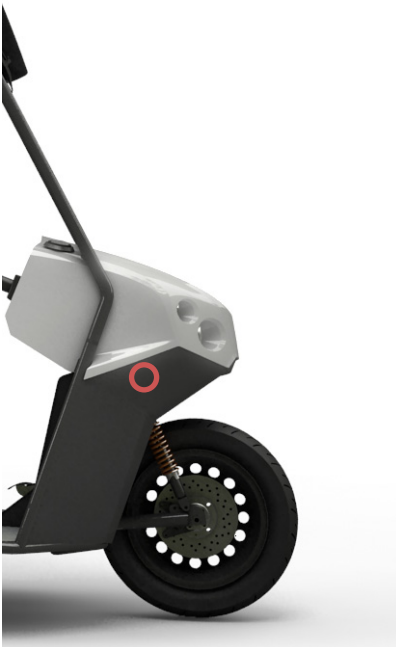
Fig. 122 Future placement of the charging inlet.
