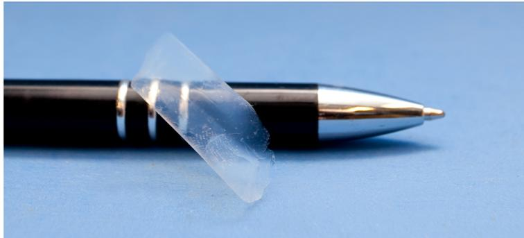
Figure 2.2: Monolithic silica aerogel. (Photo: Nina Zanders)
