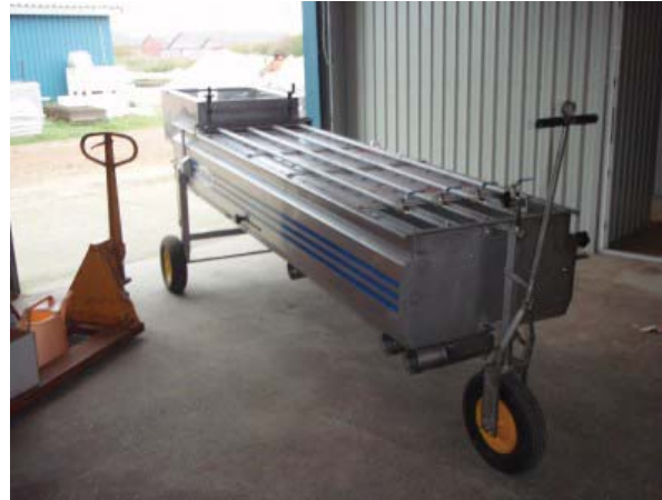
A grading machine for sorting fish of different size into different tanks
