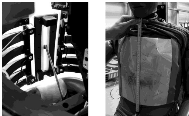
Figure 14. The left picture shows the RibEye sternal instrumentation as seen mounted in the Hybrid III chest. The RibEye system consists of six LEDs, which are optically sampled in three dimensions relative to the thoracic spine. The RibEye method of measuring allow for the standard chest sensor to be used simultaneously. The right picture shows the pressure sensitive film, which was attached to the anterior chest of the Hybrid III.
