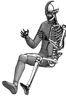
Figure 12. The THUMS HBM. Soft tissue has been removed from the left side of the body for illustration purposes. The version illustrated here is the THUMS v3.0 with refined thorax (Pipkorn and Mroz, 2008; Mroz et al., 2010 and Mendoza-Vazquez, 2012).
