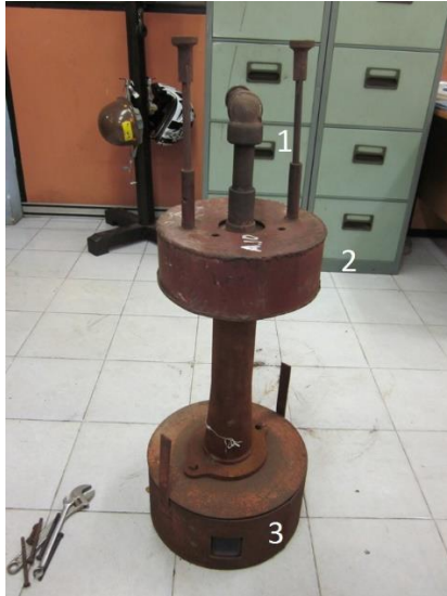
Figure 4. One of the 200 burners in the primary reformer. The fuel enters in the top (1), is pre-mixed with primary air (2) and finally the premixed fuel mixes with secondary air and combustion takes place (3).
