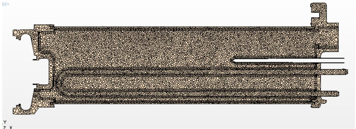
Figure 51 Plane section of 3mm base size mesh
