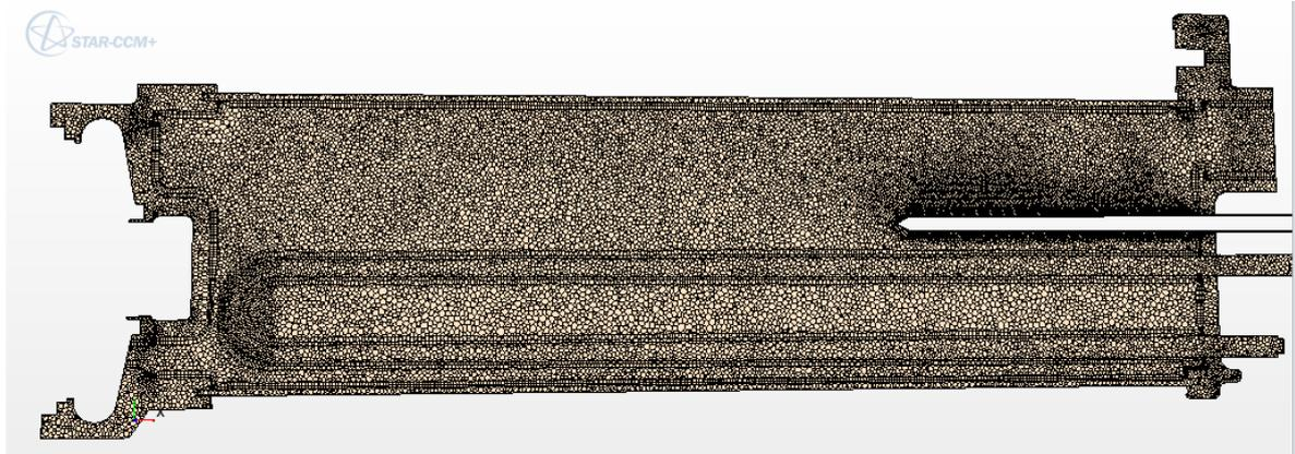
Figure 49 Plane section of 0.5 mm base size mesh
