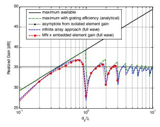
Fig. 2. Realized gain of  $32 \times 32$  element regular array of open-ended waveguides in infinite ground plane when the element spacing in H-plane is dx=0.67 $\lambda$  for different element spacings in E-plane, by different methods.
