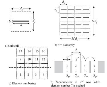
Fig. 1. Definition of a planar array of rectangular open-ended waveguides, illustrated by thick solid lines. The unit cells are illustrated by dashed squares. The lower sketches illustratess the definition of the element numbering.
