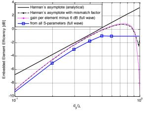
Fig. 3. Embedded element efficiency of the same 32x32 array as in Fig. 2, evaluated by different accurate and approximate methods.
