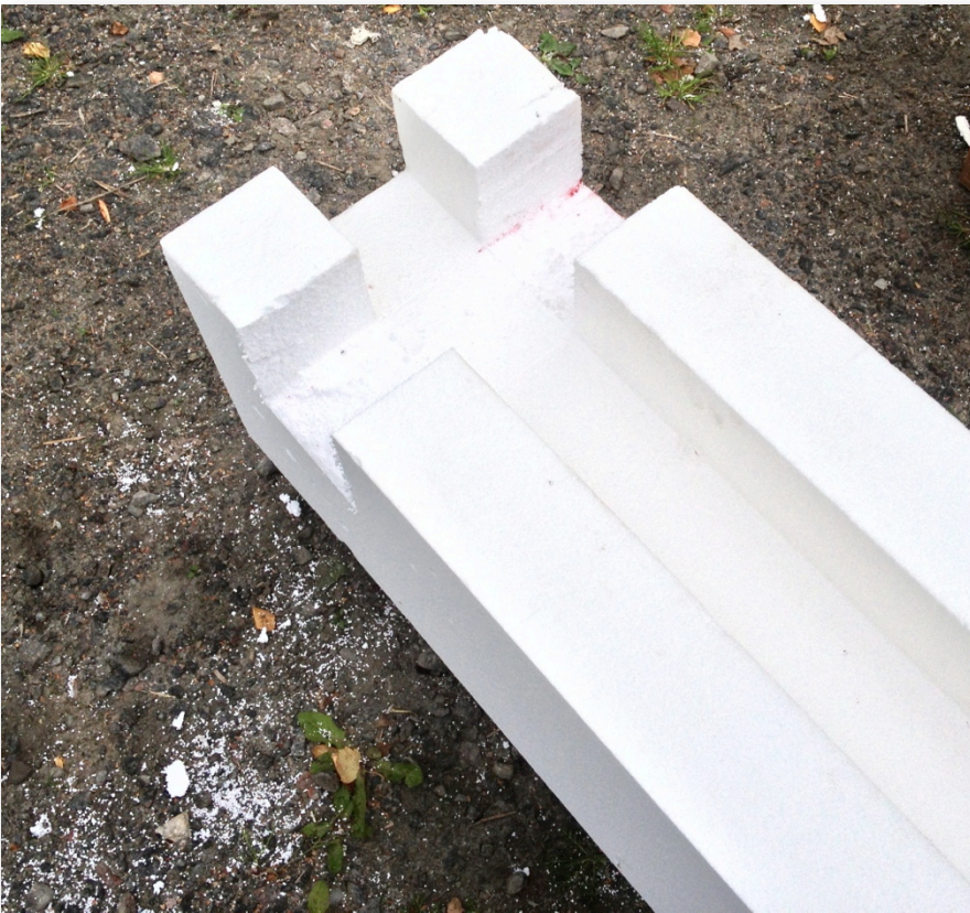
Figure 39: Styrofoam with a cut groove to fit in the corner
