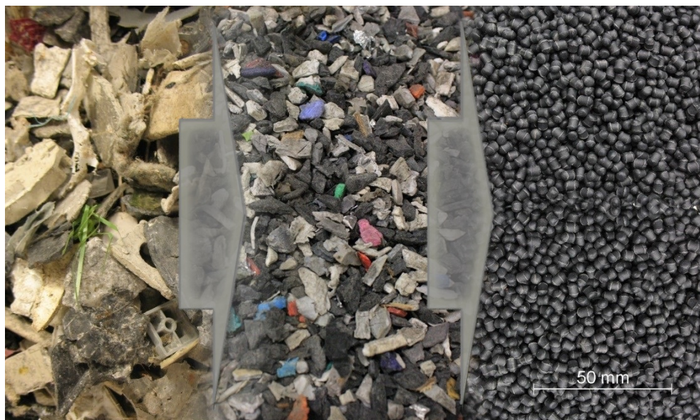
Figure 29. WEEEER granules (right) formed from melt-blending and melt-filtration of WEEE plastic flakes (left)
