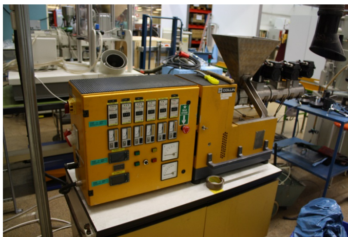
Figure 18. The single screw extruder, Collin type 132, used for melt-processing the plastics
