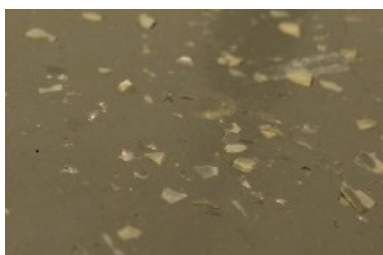
Figure 28. Photograph showing the poor material quality of a pressed WEEE (Stena 1) thermoplastics plate (before melt-filtration). The millimetre-sized particles consisted of non-thermoplastic contaminants, mainly rubbers.
