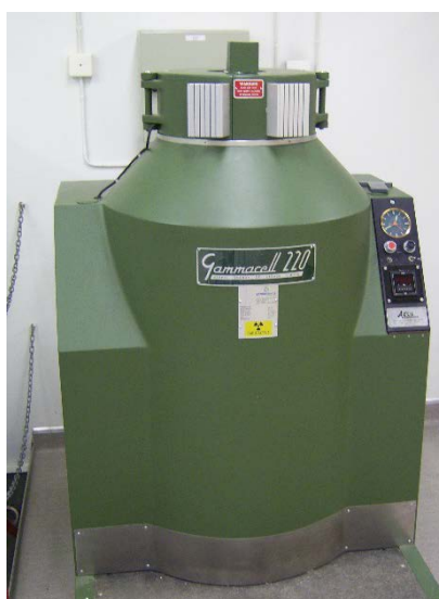
Figure 9. The gamma irradiation source (Gammacell 220) used for gamma irradiation of plastic samples
