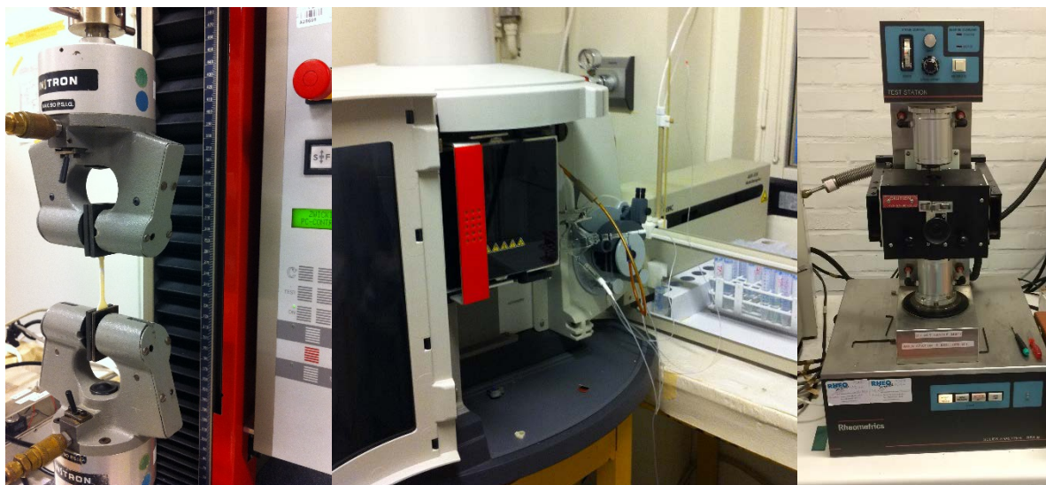
Figure 17. Equipment used for tensile testing (left), induced coupled plasma-optical emission spectroscopy (ICP-OES) (middle) and thermal testing by a dynamic mechanical thermal analysis (DMTA) machine (right)
