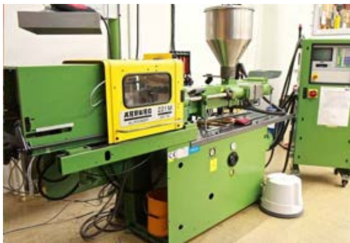
Figure 20. The injection moulding machine, Arburg Allrounder 221M 250-55, used for melt-processing the plastics
