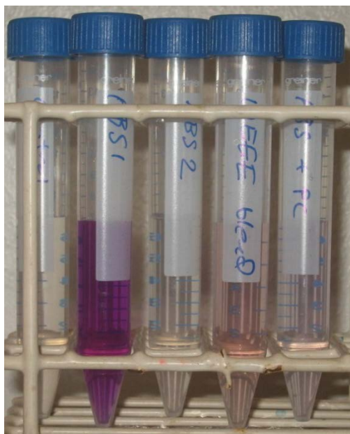
Figure 39. Hydrogen cyanide test from left to right: control sample, ABS Terluran GP-35 (purple), ABS Cyclac S157, WEEEBR, PC/ABS Bayblend FR3000. Only the purple sample indicates hydrogen cyanide anions in the sample.
