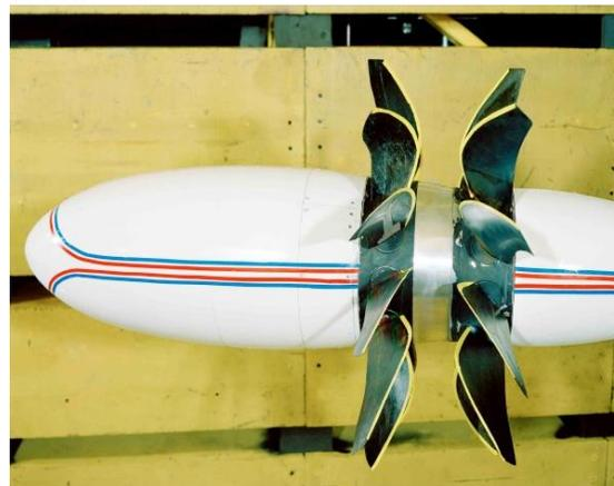
Figure 2 - The advanced forward-aft swept counter-rotating propeller concept tested by NASA during the final stages of the ATP program. Adapted from Van Zante<sup>4</sup>.
