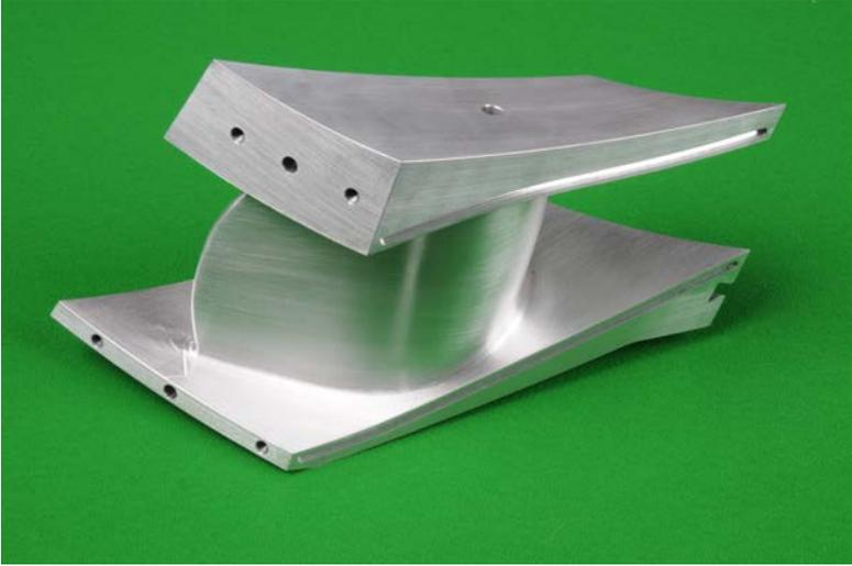
Figure B.0.3: *FACTOR ITD vane ahead of instrumentation*
