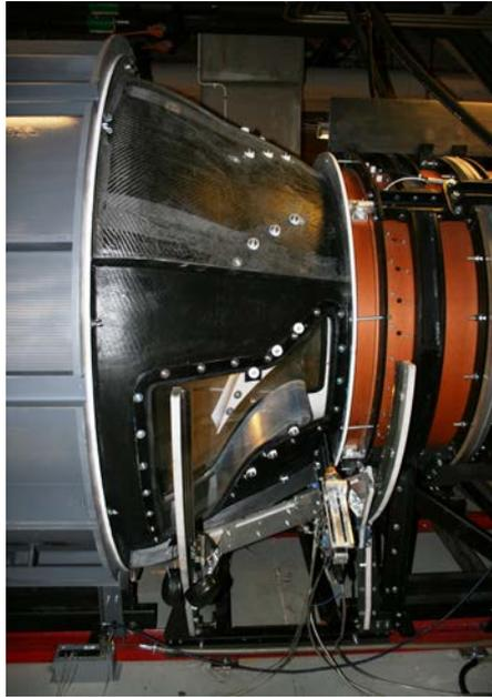
Figure B.0.1: Working section of Chalmers LSLS Turbine Facility with traverse system in view
