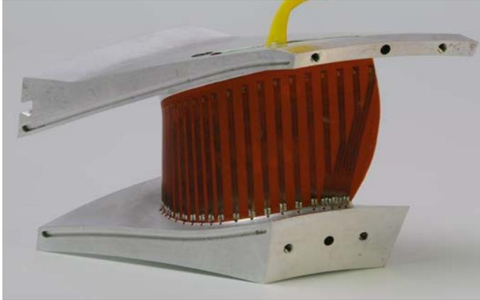
Figure 4.2.5: *ITD vane instrumented with TFHFGs at 90% height*
