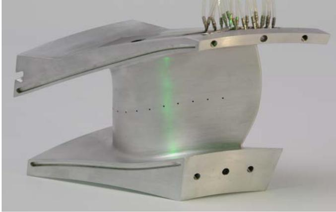
Figure 4.2.2: *ITD vane instrumented with static pressure tappings at 50% height*
