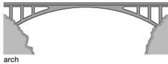
Figure 3.2 Arch bridge (Billington P. 2015)
