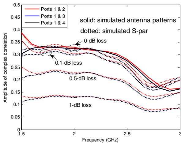
Fig. 3. Correlation from simulated S-parameters and antenna patterns with various cable insertion loss.
