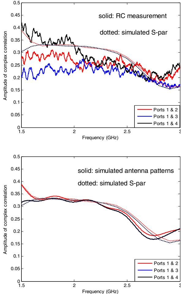
Fig. 2. Bowtie correlation. (upper) RC measured correlation vs correlation calculated from S-par; (lower) correlation calculated from S-par vs correlation calculated from antenna pattern.
