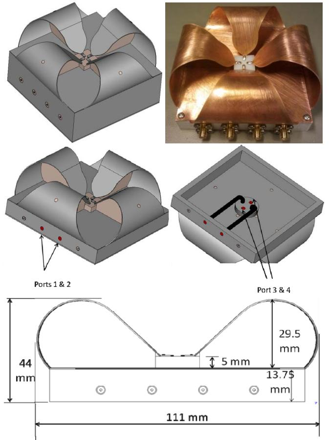
Fig. 1. Photo and drawings of the Bowtie antenna [10].
